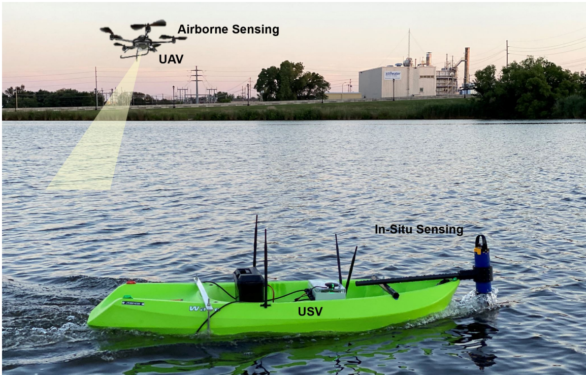
Figure 2: UAS for water quality monitoring
