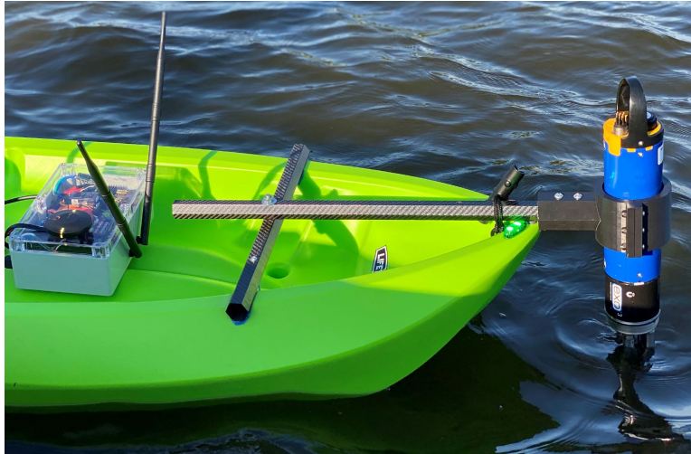
Figure 42: Front position of the Sonde
