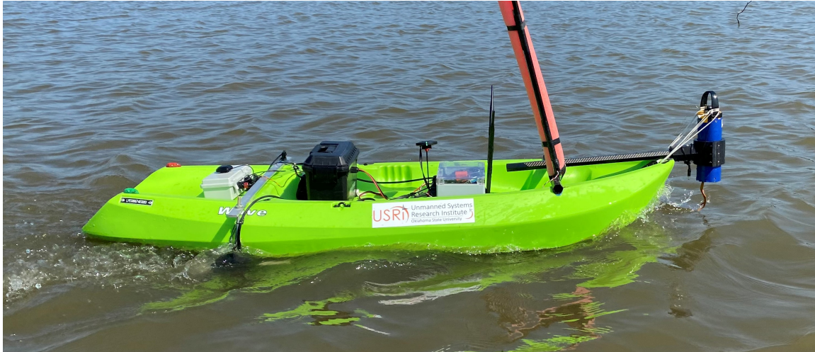
Figure 81: MANUEL's Sonde broke during an AUTO mission
