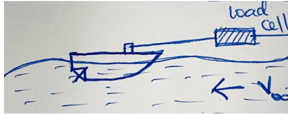
Figure 14: Estimating the total drag on MANUEL
