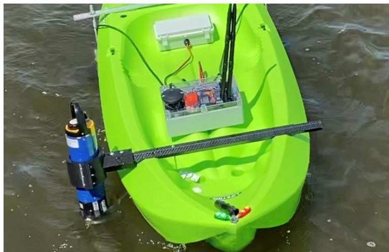
Figure 41: Side position of the Sonde
