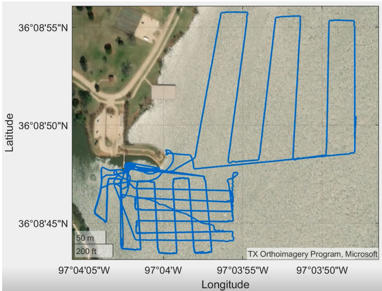
Figure 48: MANUEL's different auto mission paths during test at Boomer lake
