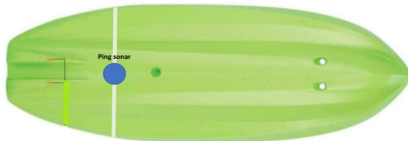
Figure 43: Bottom view showing Ping sonar placement
