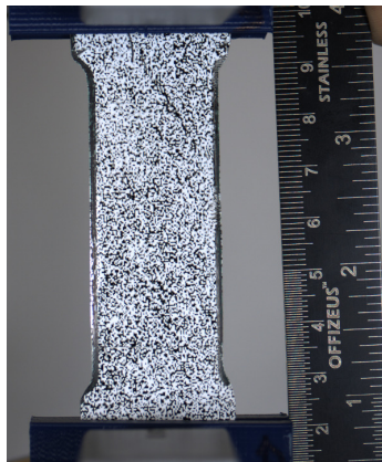
Figure 15: Calibration image recorded before the test.
