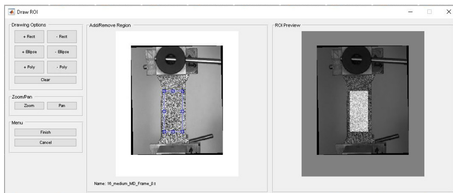
Figure 18: ROI drawn on the specimen in Ncorr software.
