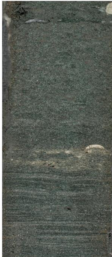
Figure 22. – Siltstone and sandstone facies of the Gordo Formation (Marine Tuscaloosa shale) from MPC 10-4 well. A) Graded muddy siltstone lithofacies, 3205 ft measured depth, has soft
