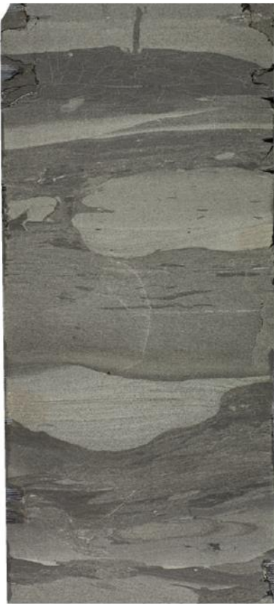
Figure 22. – Siltstone and sandstone facies of the Gordo Formation (Marine Tuscaloosa shale) from MPC 10-4 well. A) Graded muddy siltstone lithofacies, 3205 ft measured depth, has soft
