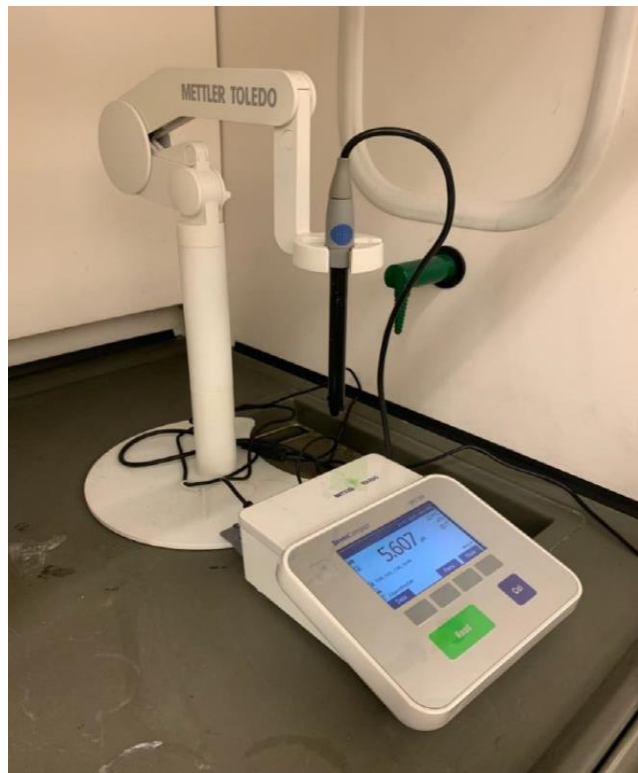
Figure 3. 7. SevenCompact pH meter S220 used for pH and ionic strength measurements
