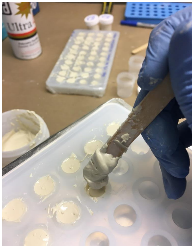
Figure 3. 3. Molding geopolymer slurry into half-inch diameter spheres
