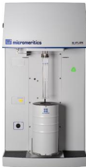
Figure 3. 11. 3 Flex Surface Characterization Analyzer (Micromeritics, Norcross, GA)
