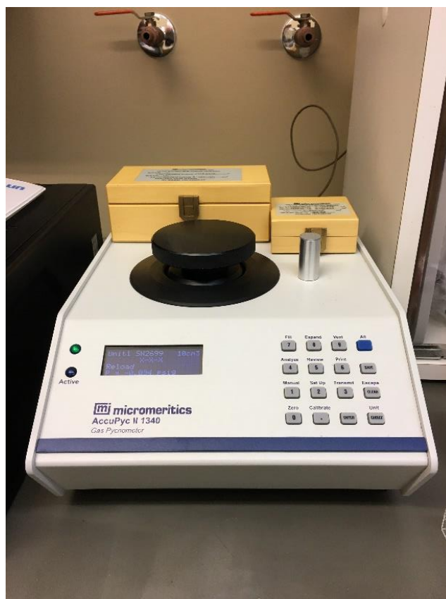
Figure 3. 10. Gas displacement pycnometry system, AccuPyc II 1340 (Micromeritics, Atlanta, GA)
