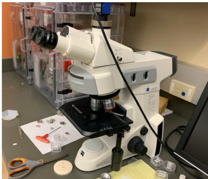
Figure 3. 4. Carl Zeiss' AxioLab A1 Modular, upright Optical Microscope for Materials Science (Carl Zeiss Microscopy, LLC, White Plains, NY)
