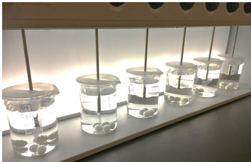
Figure 5. 1. Agitator setup of six having triplicate solutions of each batch adsorption test. Two sets of adsorption experiments can be run at the same time. (Velp Scientifica, Bohemia, NY)
