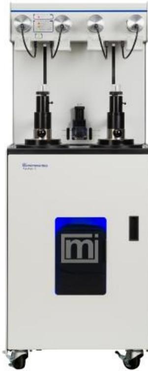
Figure 3. 12. Autopore V, Mercury Intrusion Porosimetry (MIP) (Micromeritics, Norcross, GA)
