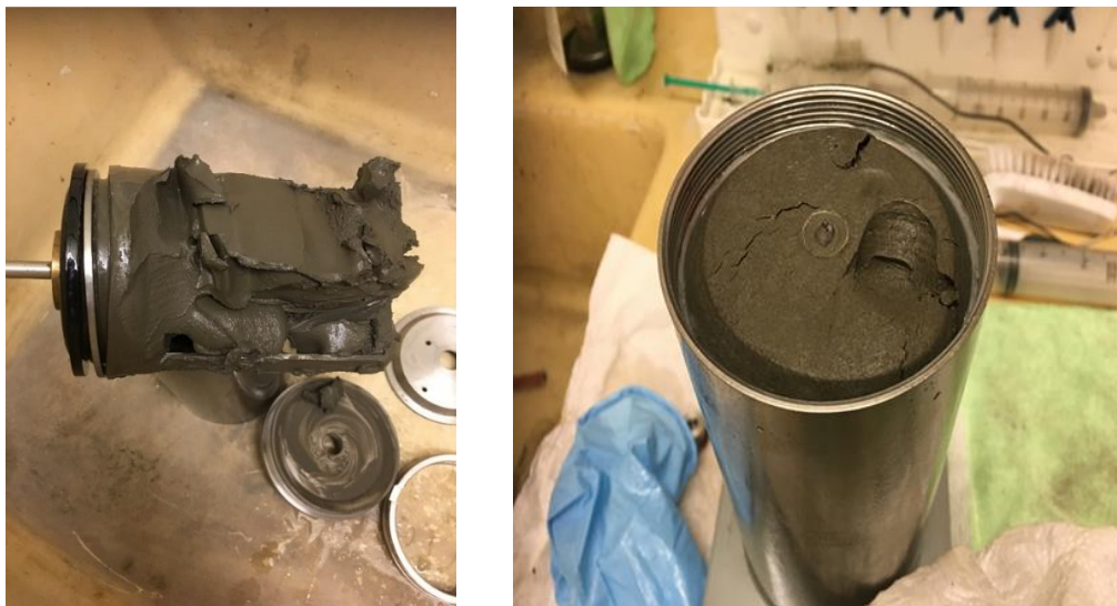
Figure 4.1 The cement after it has reached 80 Bc in the consistometer
