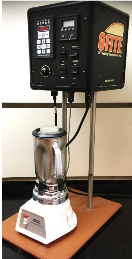
Figure 3.1 OFITE Model 20 cement mixer
