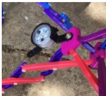
Figure 4. Attached LED light – LED light screwed onto the junction point of the Hoberman Sphere with the black plastic clamp.
