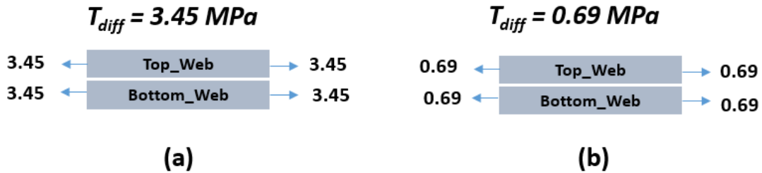
Figure 5.15: Cases with two different web tensions, For (a) T_{diff} = 3.45 \text{ MPa} ; (b) T_{diff} = 0.69 \text{ MPa}
