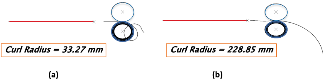
Figure 6.11: MD curl in the laminated web for (a) Model-II; (b) Model-IV
