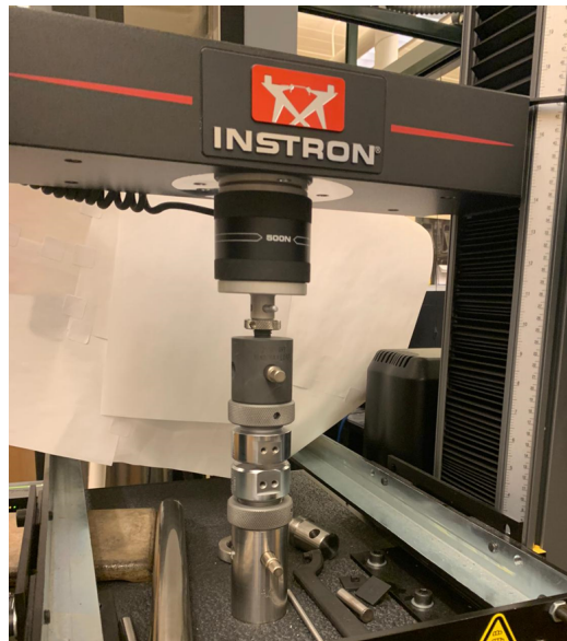
Figure 14.7: Setup of creep test on Instron tensile machine
