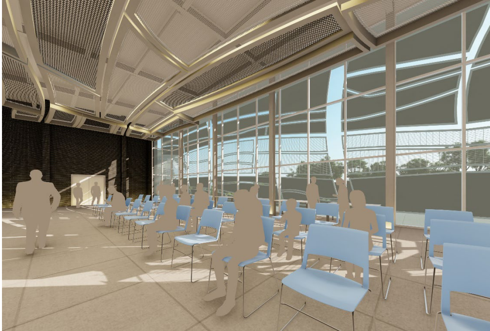
Interior render of the Demonstration Space with the metal mesh system applied to the façade and ceiling.
