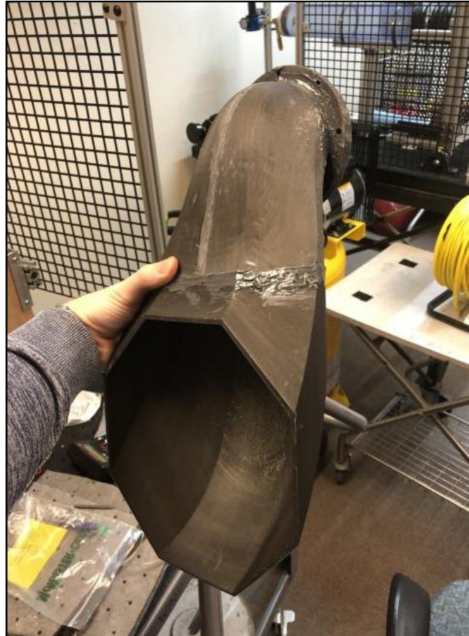
Figure 22: 6" Octagonal Inlet (Iteration 1)
