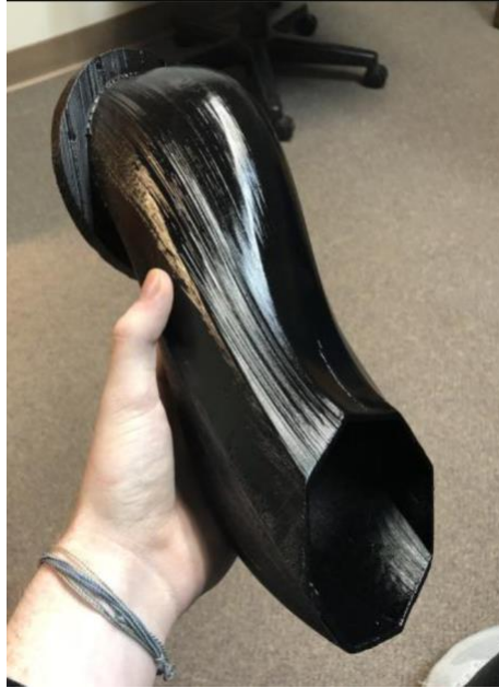
Figure 31: 6" Octagonal Inlet (Iteration 2)
