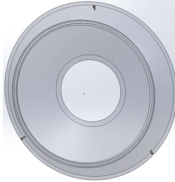
Figure 7: CAD Model of Cowling with Screw Placement
