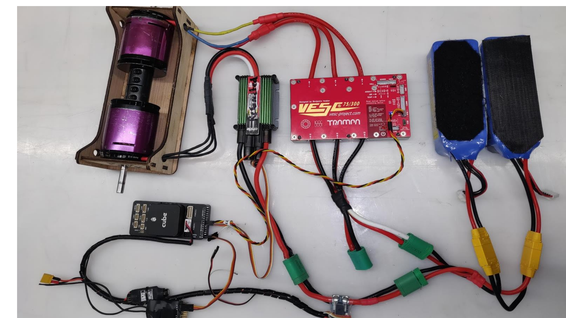
Figure 5: Experimental apparatus for VESC testing, utilizing a motor/generator pair, LiPo batteries, a BLDC motor driver, and a Pixhawk for logging power data.
