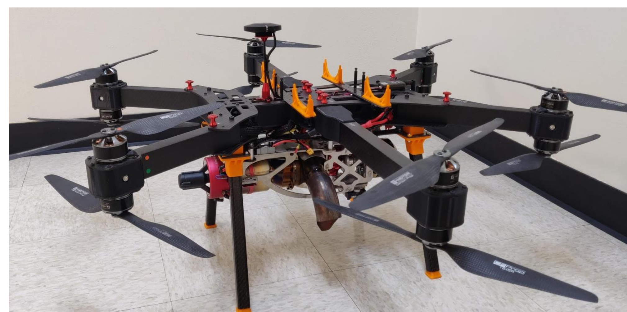
Figure 1: X-Fold Dodecaopter outfitted with turbo-electric power system.
