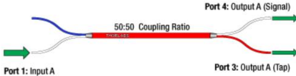
Figure 3-2. ThorLabs' 10202A-50-FC 50:50 Splitter.
