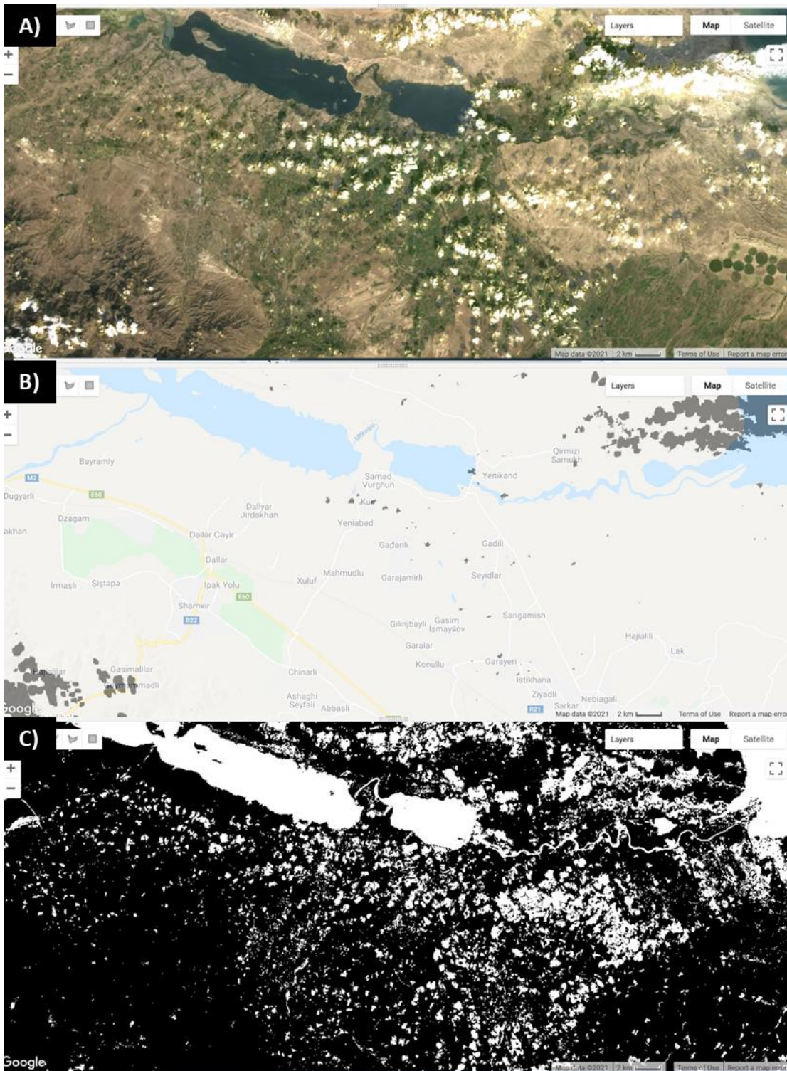
Figure 9. This figure shows the undetected cloud/cloud shadows in the pixel_qa cloud mask around the Yenikend Reservoir, Azerbaijan. (A) True -color Landsat 8 image of Path/Row set 4 acquired on October 22, 2019. (B) The pixel_qa cloud mask, where the clouds detected are represented by grey areas. (C) Final OPC water map containing cloud/cloud shadows present in the scene but omitted from the pixel_qa cloud mask.
