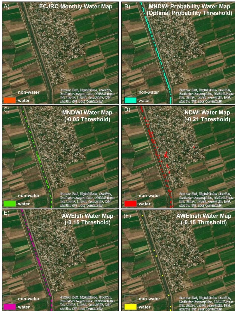
Figure 9: Compares the ability to detect the Upper Garabakh Canal, Azerbaijan, between the selected water indices, the ECJRC Monthly History water map, and the MNDWI probability water map, using the OPC value method. The thresholds chosen for the selected water indices were determined by applying the lowest potential threshold value for each water index, as listed from previous studies. (A) shows a true-color image of the Upper Garabakh Canal. (B) Canal water detected by the MNDWI probability water map. (C) Canal water identified by the MNDWI water index (-0.05 threshold). (D) Canal water identified by the NDWI water index (-0.19 threshold). (E) Canal water detected by the AWEIsh water index (-0.15 threshold). (F) Canal water identified by the AWEInsh water index (-0.15 threshold).
