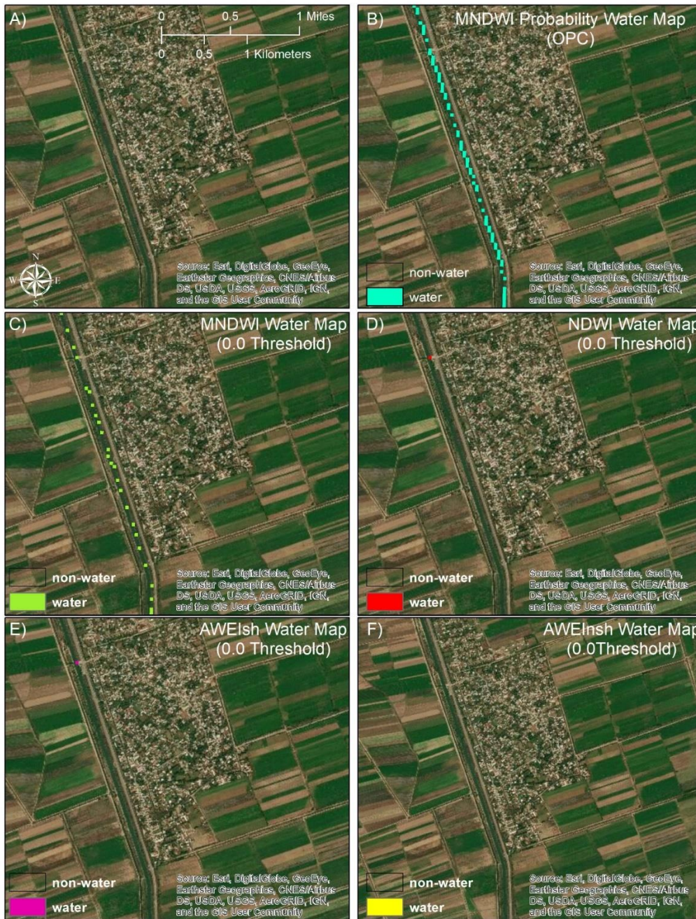
Figure 8: Compares the ability to detect the Upper Garabakh Canal, Azerbaijan, between the selected water indices and the MNDWI probability water map, using the OPC method. The thresholds chosen for the selected water indices were determined by applying a threshold value of zero for each water index. (A) shows a true-color image of the Upper Garabakh Canal. (B) Canal water detected by the MNDWI probability water map. (C) Canal water identified by MNDWI water index (D) Canal water identified by the NDWI water index (E) Canal water detected by the AWEIsh water index. (F) Canal water identified by the AWEInsh water index.
