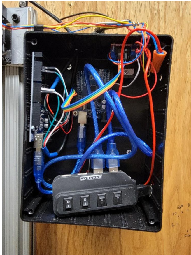
Figure 13: Two Arduino boards operating to control motor and record sensor data
