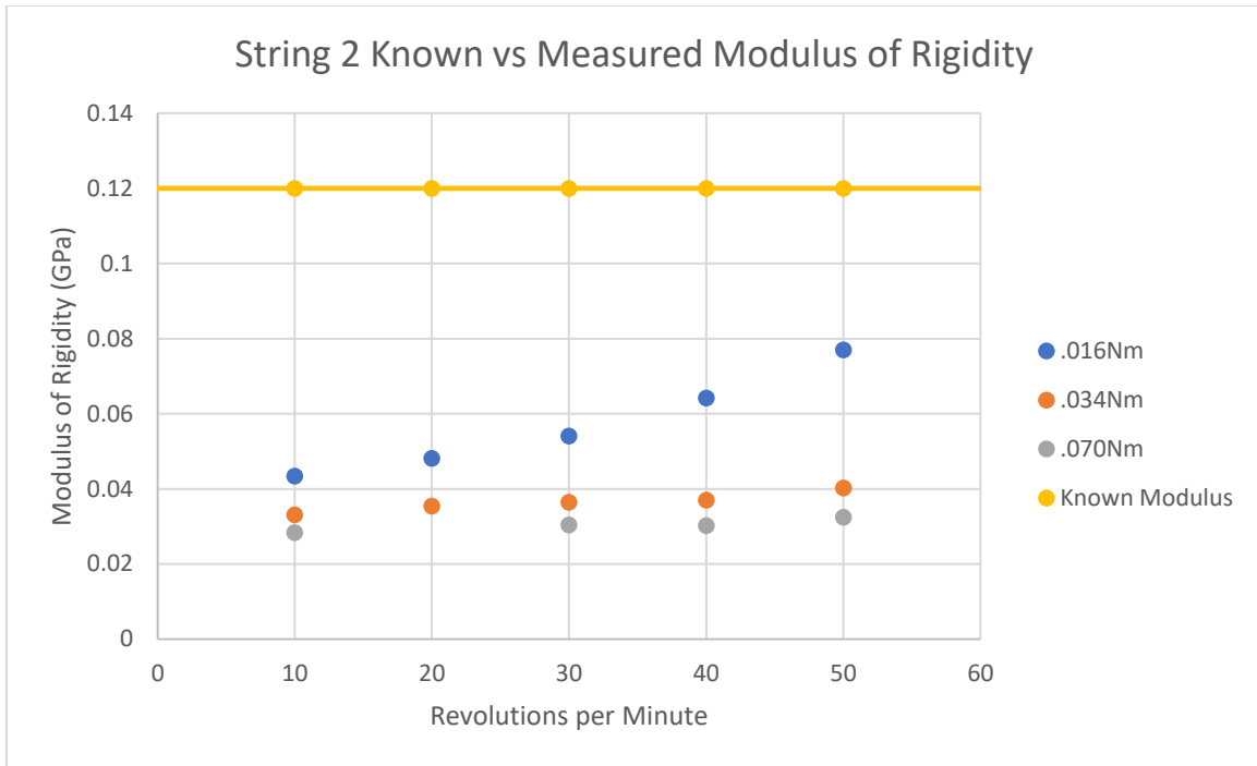
Figure 19: String 2 modulus of rigidity vs revolutions per minute with the inclusion of torque from friction
