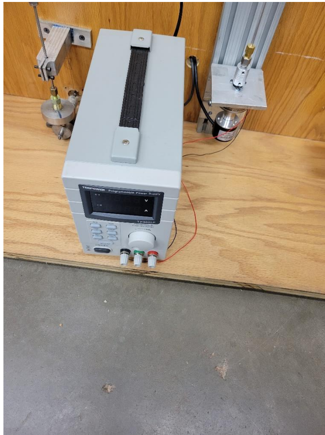
Figure 12: Power supply to the brake at bottom of string
