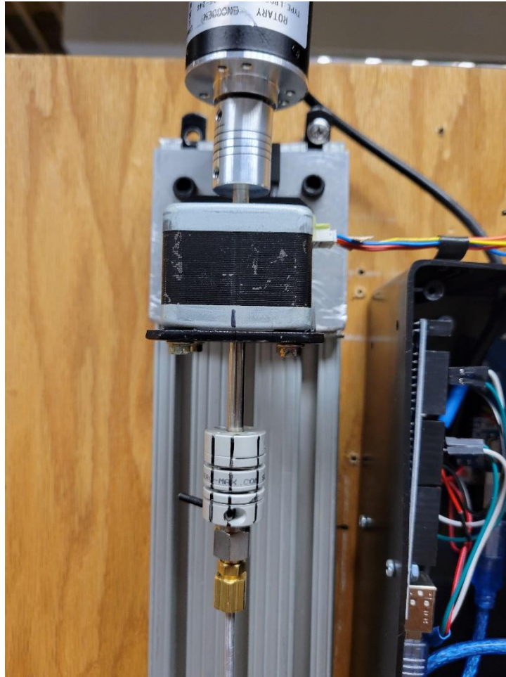
Figure 10: Top sled containing rotary encoder and stepper motor
