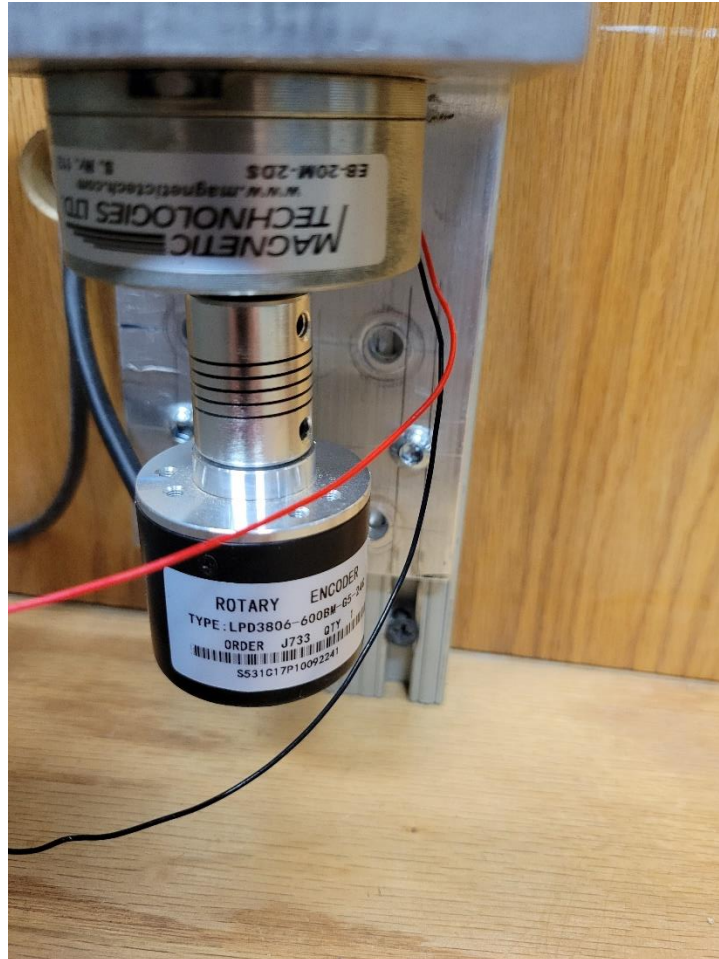
Figure 11: Brake and bottom rotary encoder
