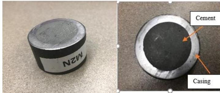
**Fig. 5-15—Specimen 1-inch × 1-inch after polishing.**
