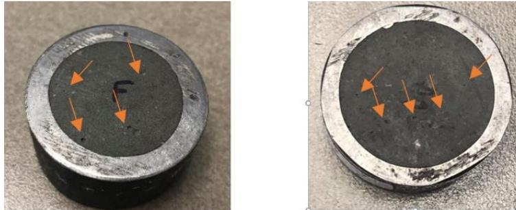
**Fig. 6-25—Bubbles appear in the cement surface after cured if tested before hardening.**
