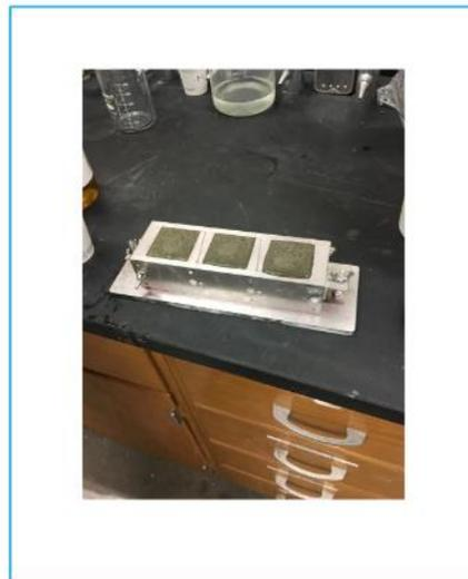
**Fig. 5-4—Cement molds with cement.**
