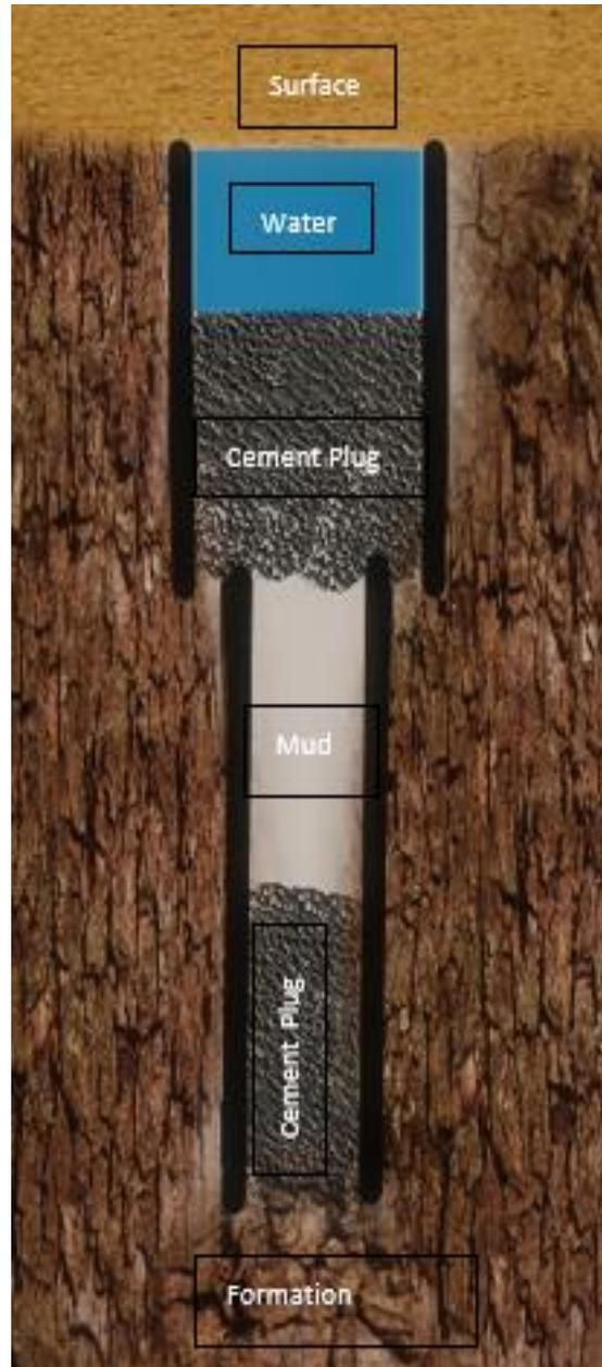
Fig. 3-6—Sketch of a cement plug.
