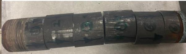
**Fig. 5-13—Specimen cut into 1-inch section**
