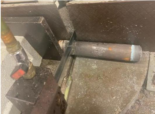
**Fig. 5-14—Specimen prepared for mechanical cutting.**
