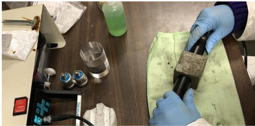
Fig. 5-5—Ultrasonic measurement at the center of the cement cube.
