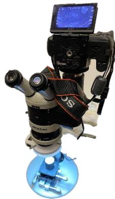
**Fig. 5-18—Microscope attached to a high-resolution camera.**
