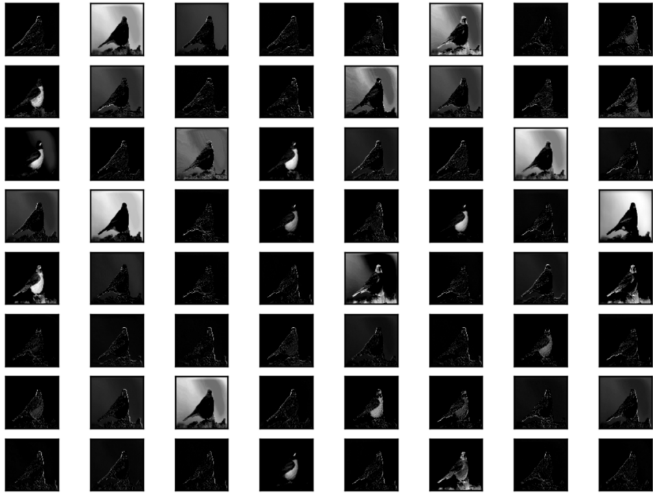
Fig. 1.29 - Example feature maps output from the first convolutional layer of a trained 16-layer convolutional neural network (Brownlee, 2019).
