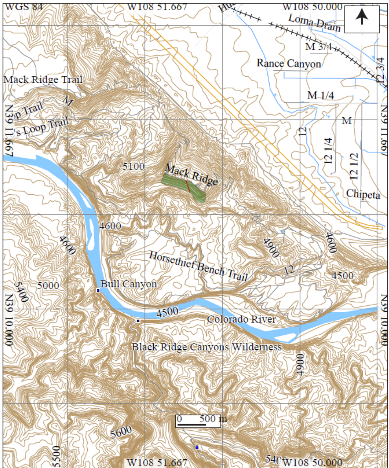
Figure 1-20A: Mack Ridge study area. Green highlight indicates extent of the outcrop reconstruction mapped using UAV (Unmanned Aerial Vehicle) photogrammetry. The location of the measured section traverse is indicated in red line. The exposed side of Mack Ridge outcrop analyzed within the Burro Canyon Formation includes the wall perpendicular to the paleoflow.
