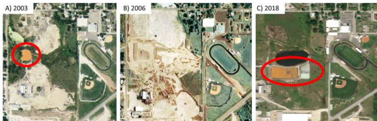
Figure 2.4: Site in Commerce, OK, having undergone substantial land modification preventing evaluation of natural evolution of trace metal changes A) Highlighting Cactus Collapse B) Site construction C) Highlighting Southeast Commerce passive treatment system
