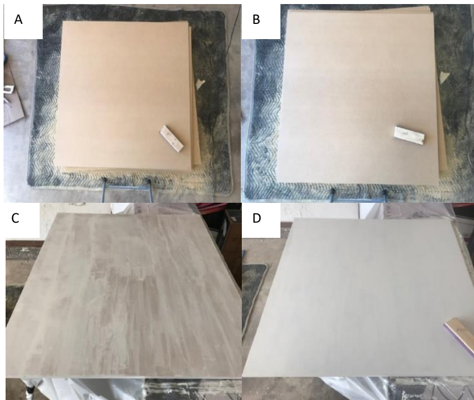
Figure 5.1 Calibrated panels in development, (A) after being sanded with 80-grit (B) and 150-grit sandpaper, (C) application of a single coat of primer, and (D) multiple coats of primer and a final sanding with 220-grit sandpaper.
