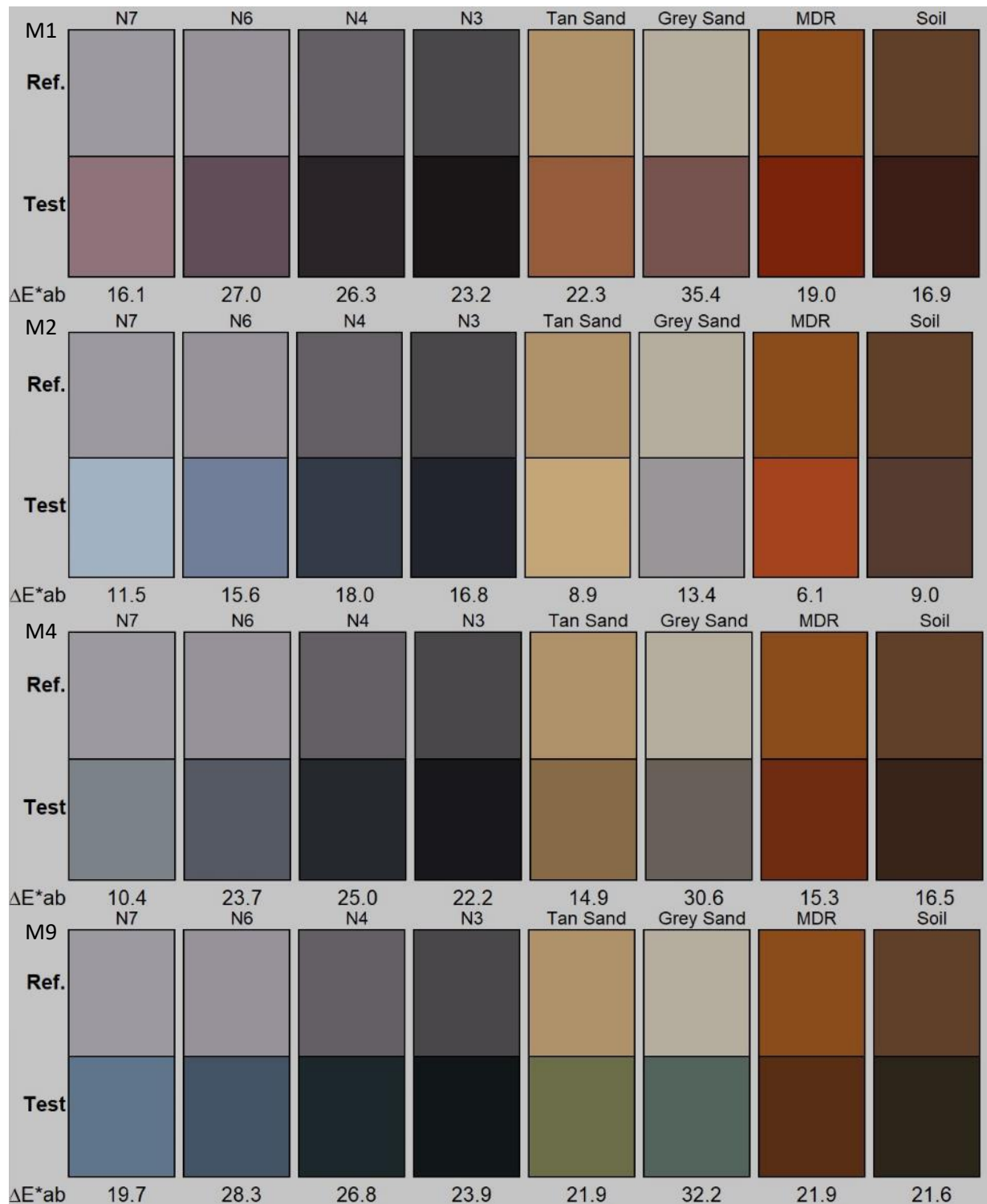
Figure 5.5 L^*a^*b^* colors of Munsell identified reference (Ref.) panels (e.g., N7 - calibrated and Tan Sand (Tsand) - natural) and those produced from M1, M2, M4, and M9 (Test) displaying the calculated color difference (e.g., \Delta E ) for each of the panels examined.
