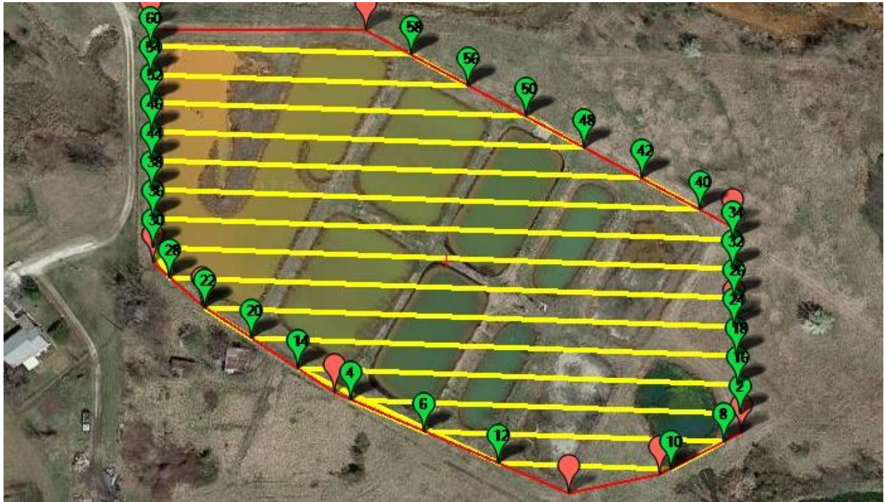
Figure 2.2 Example sUAS flight path (yellow lines) used for MS image collection, with waypoints (green numbered markers), and the mission extent (red polygon).
