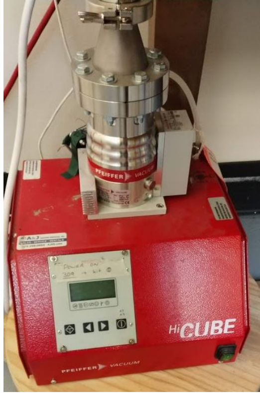
Figure 4 - Pfeiffer HiCube 80 Eco vacuum pump
