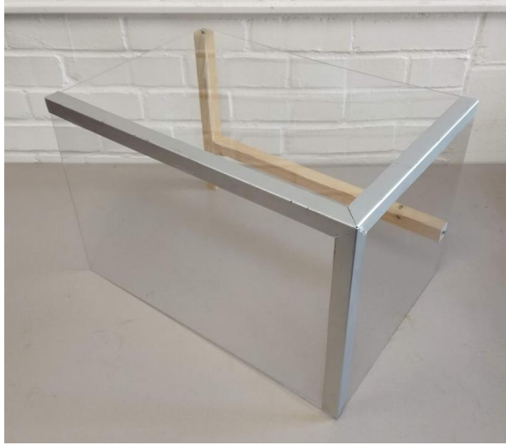
Figure 12 - Blast Shield, which sits around the camera and viewport
