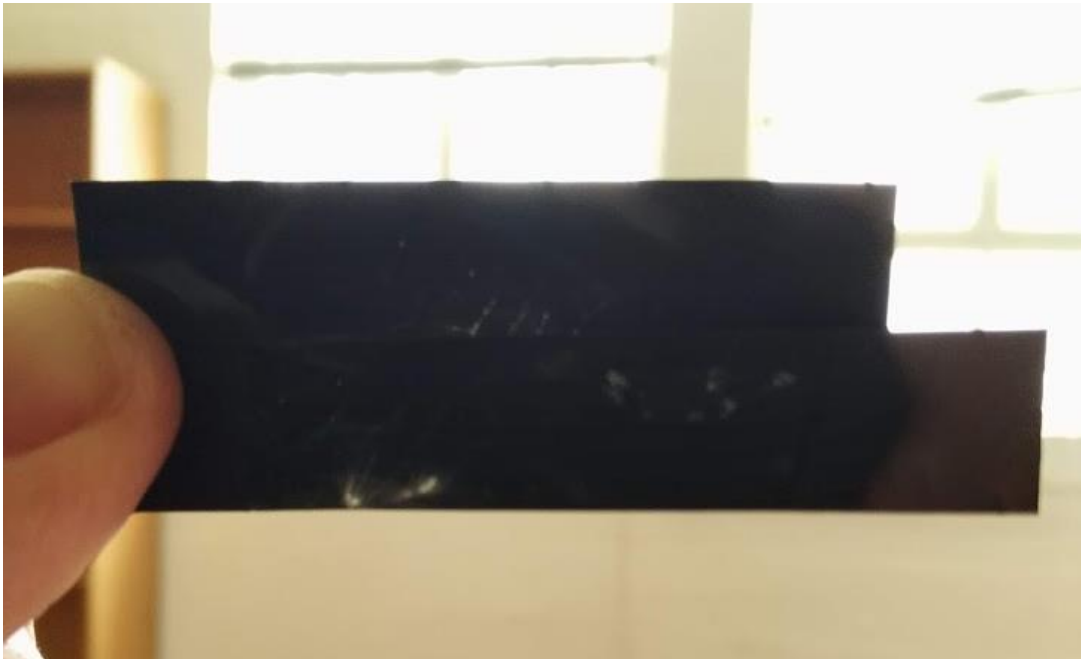
Figure 42 - Graphene/polymer nanocomposite samples, defects showing
