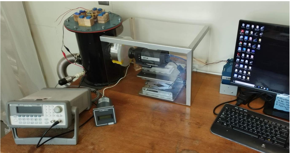
Figure 5 - Experimental setup (left to right): function generator, vacuum chamber, infrared camera, desktop computer
