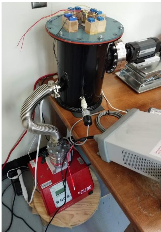
Figure 3 - Vacuum chamber, connected to vacuum pump
