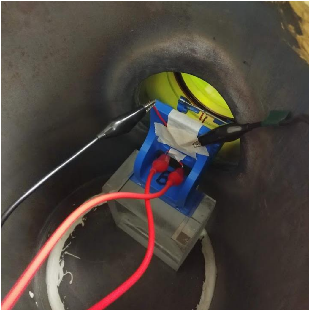
Figure 23 - Sample stage mounted inside vacuum chamber
