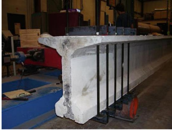
(a) Beam after steel repair
