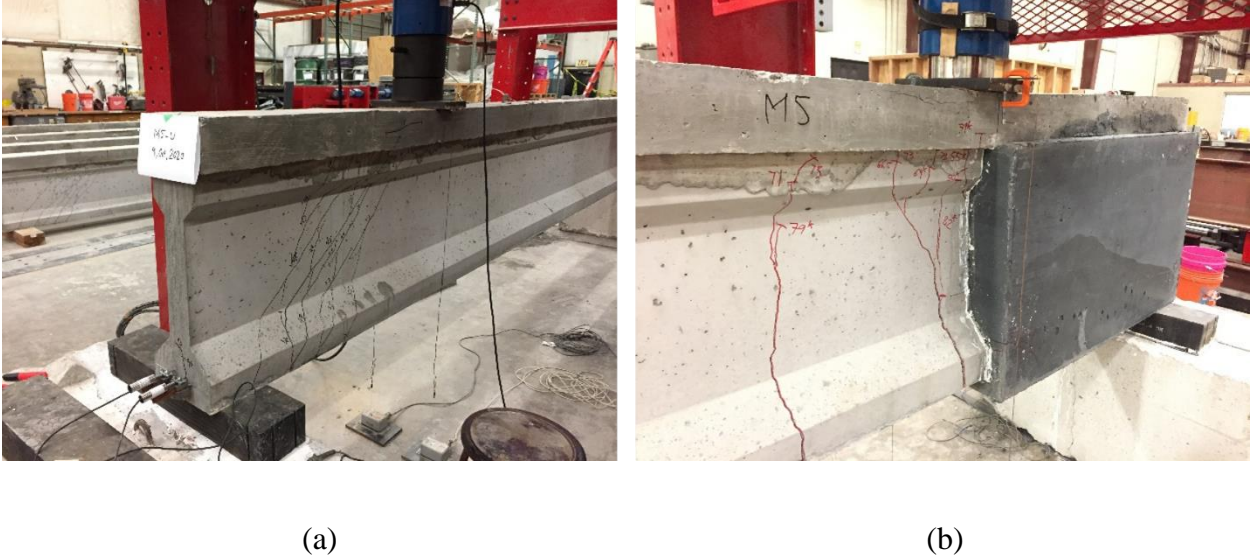
Figure 4.21: (a) Beam M5-U after the initial test and (b) beam M5-R after the final load test
