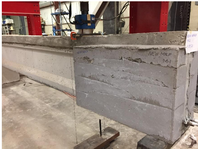
Figure 4.2: Beam M1-R during the load test
