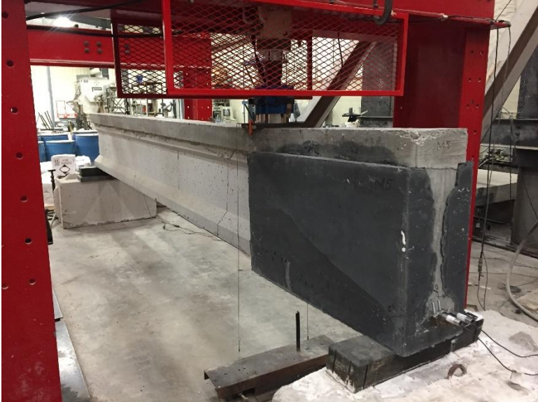
Figure 4.22: Beam M5-R during the load test
