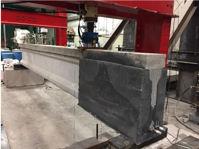
Figure 4.27: Beam M6-R during the load test
