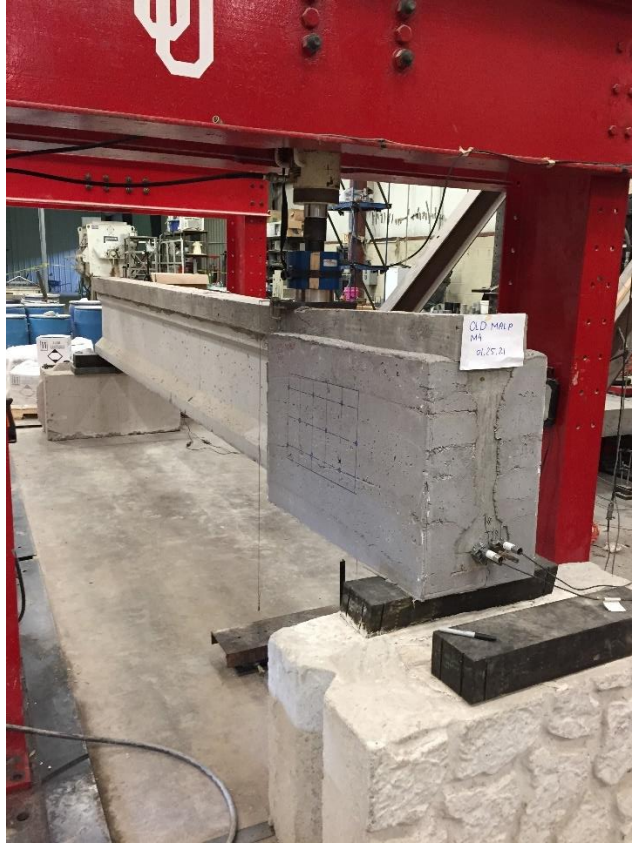
Figure 4.7: Beam M4-R during the load test
