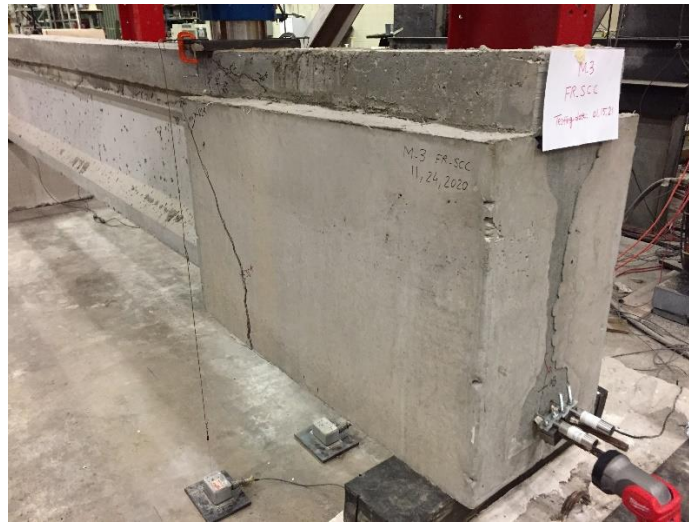
Figure 4.17: Beam M3-R during the load test
