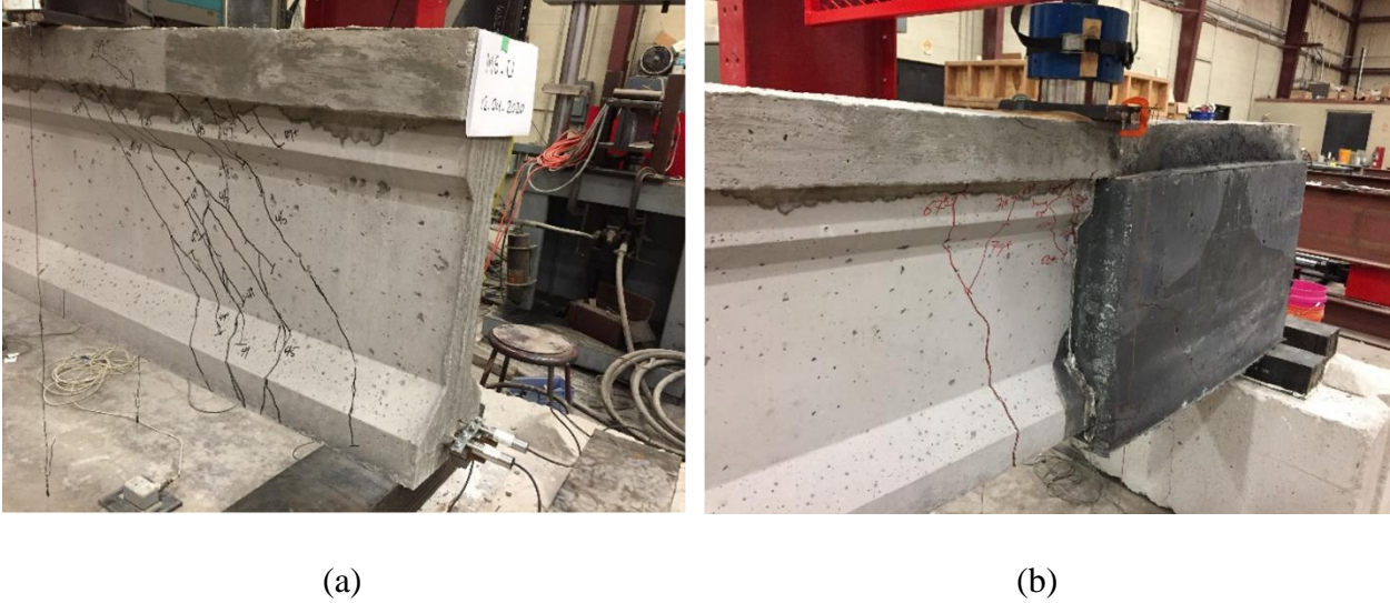
Figure 4.26: (a) Beam M6-U after the initial test and (b) beam M6-R after the final load test
