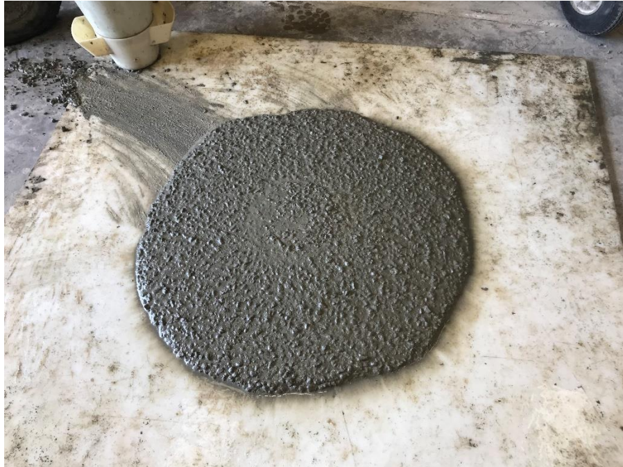
Figure 3.17: FR-SCC flow for the slump measurement
