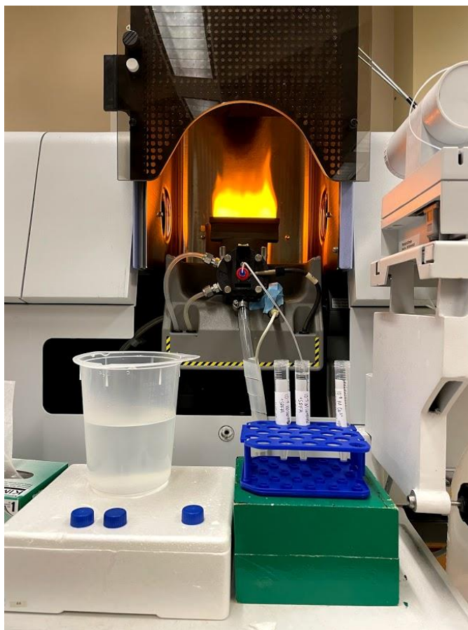
Figure D2. Atomic Absorbance Spectrometer used to measure absorbance of Cu in the solution used to determine the amount of free Cu in solution.
