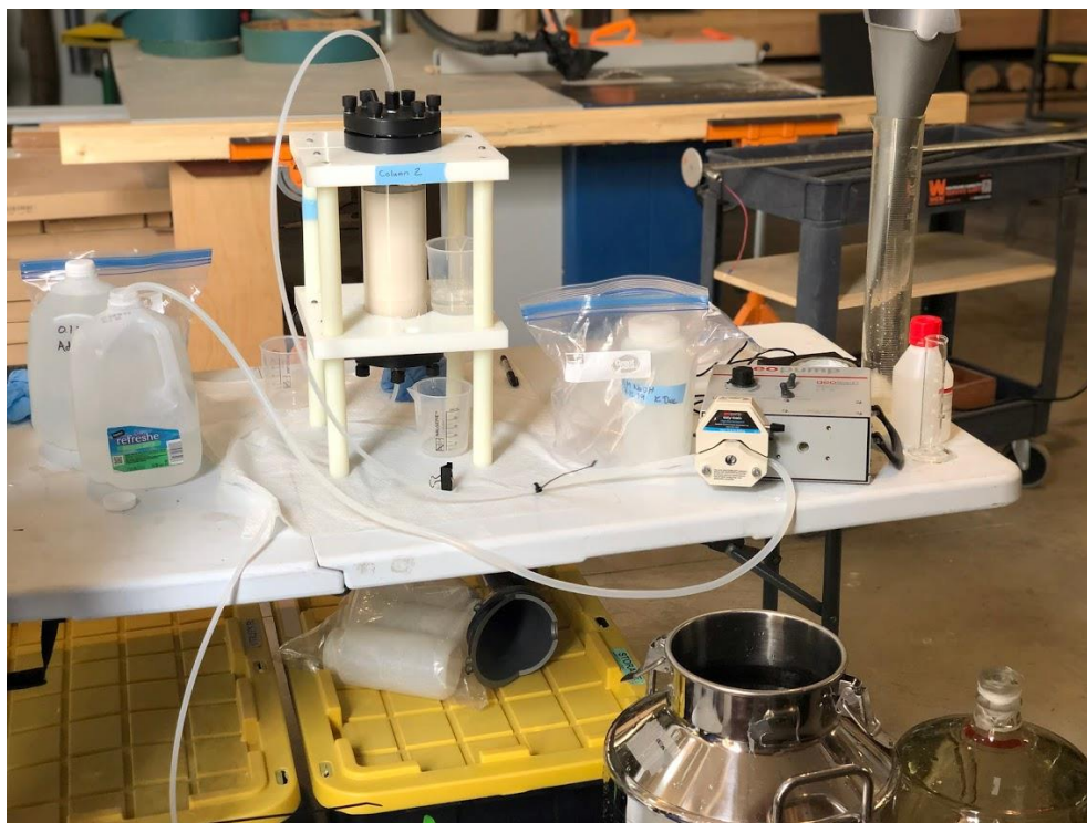
Figure C1. Set-up for an in-line approach for H^+ saturated FA isolates for 50 L in 5cm column.
