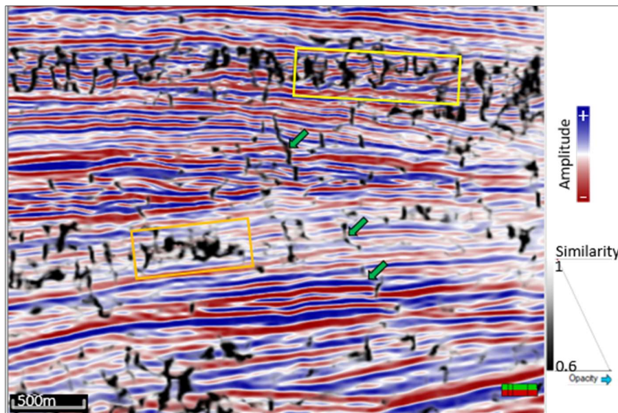
Figure 1. 17 – Vertical section with the amplitude volume (red-white-blue color) corendered with similarity attribute. It is possible to see that low similarity values will be associated with faults (green arrows), chaotic deposits (yellows box), and seismic noise (orange box).
