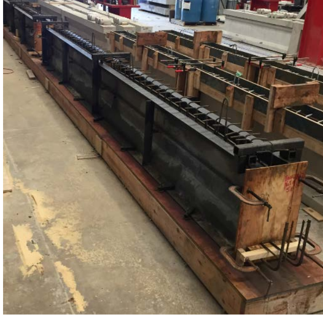
Figure 3-18: Specimens Ready for Casting
