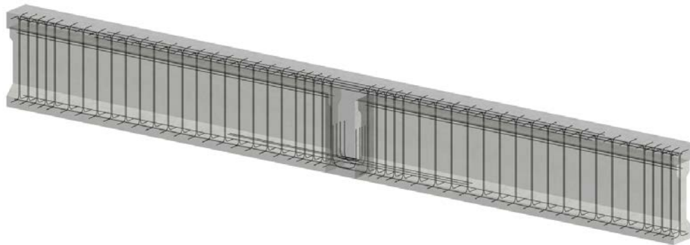
Figure 3-12: 3-Dimensional Representation of Full-Length Specimen Steel Reinforcement
