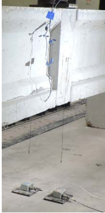
Figure 4-3: Wire Potentiometer Setup
