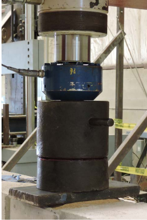
Figure 4-1:Hydraulic Ram, Load Cell, Spacer, and Metal Plate Setup
