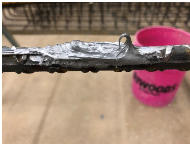
Figure 3-27: Room-Temperature-Vulcanizing Silicone (RTV) Covering Strain Gauge
