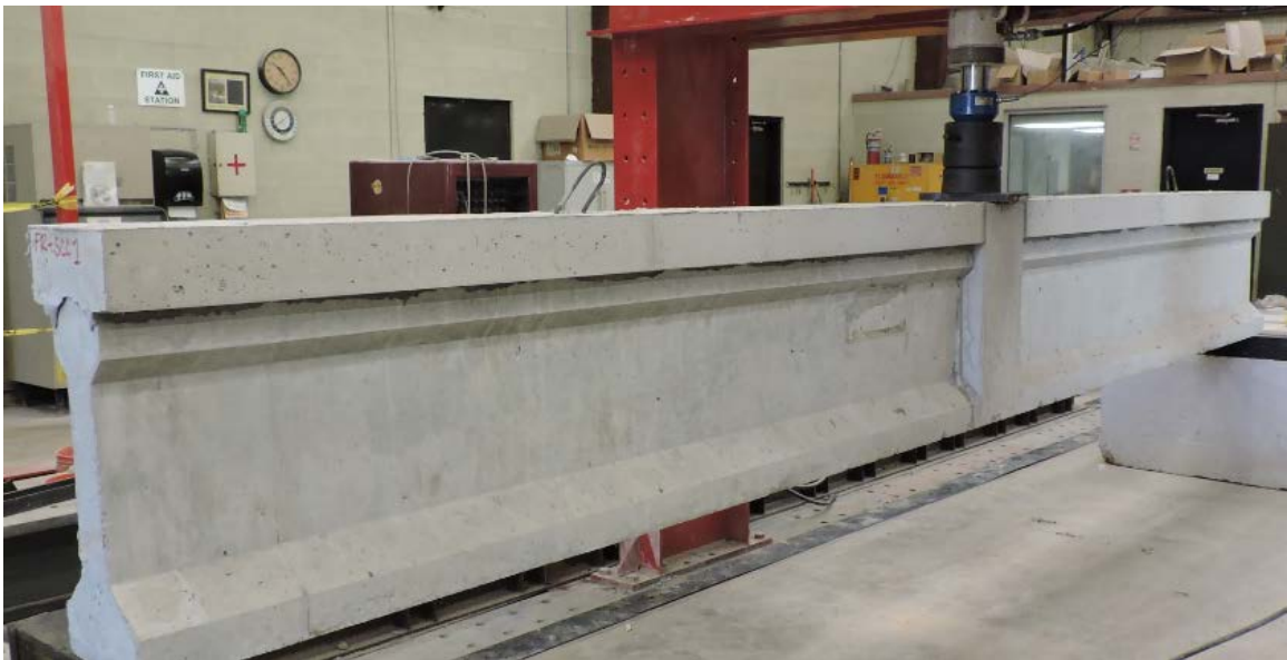
Figure 4-28: Initial Setup Before Testing for Girders to Be Repaired
