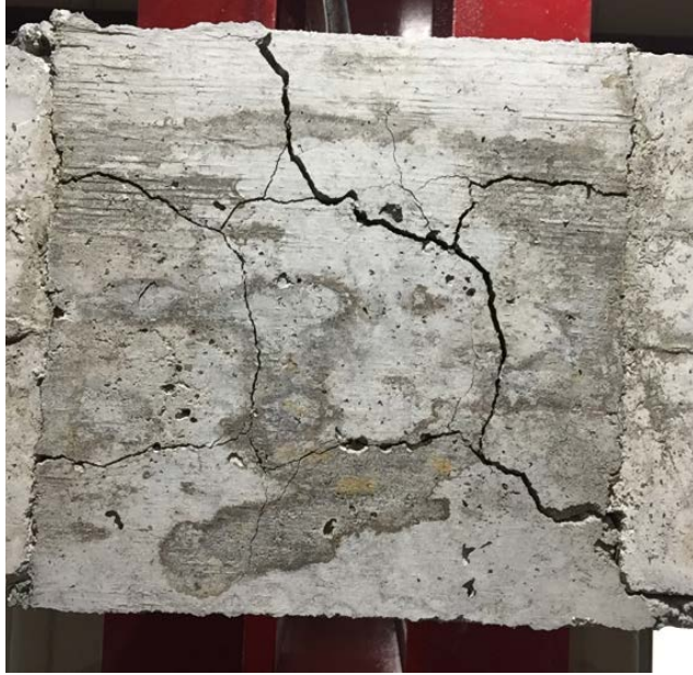
Figure 4-39:R1-FRSCC Bottom Joint Face Initial Cracking
