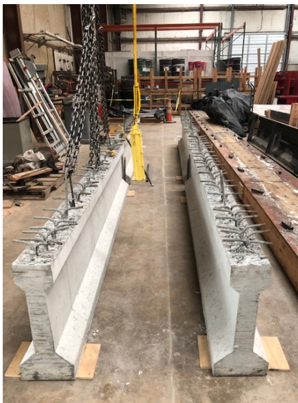
Figure 3-22:Half-Length Girder Specimens After Moist Cure
