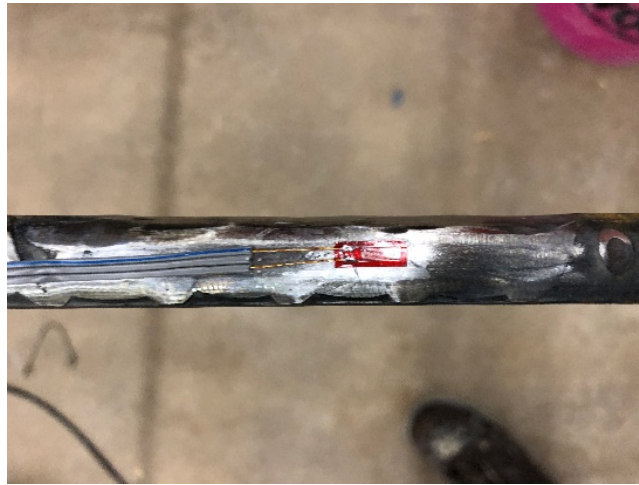
Figure 3-26: Strain Gauge Glued to Longitudinal Reinforcement
