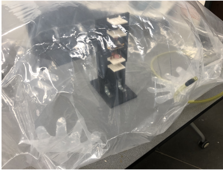
Figure 4.25: Entire mounting structure, Galinstan-filled syringes, and filter placed within a Nitrogen-filled sealed glove bag.
