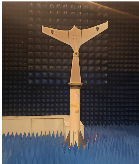
Figure 5.38: Mounting configuration for measuring underside of UAV
