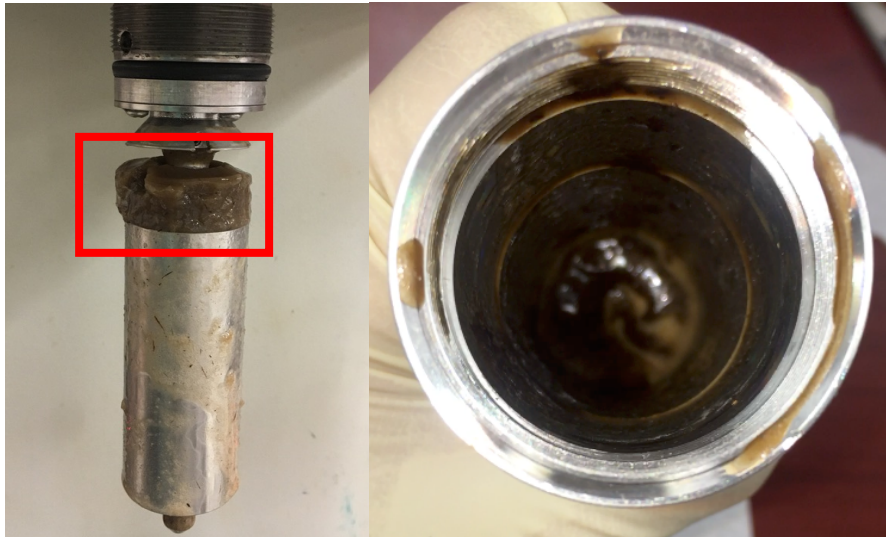
Figure 24. A gelled portion of samples placed on top of the rheometer bob after 400°F test (left), and a portion of mud sample with a high concentration of burn Cedar Fiber in the bottom of the sample cup (right).
