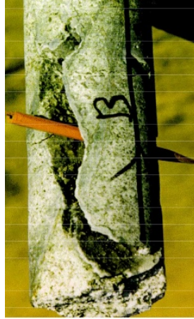
Figure 6. Large fracture in a geothermal well core sample (Blankenship, 2016)
