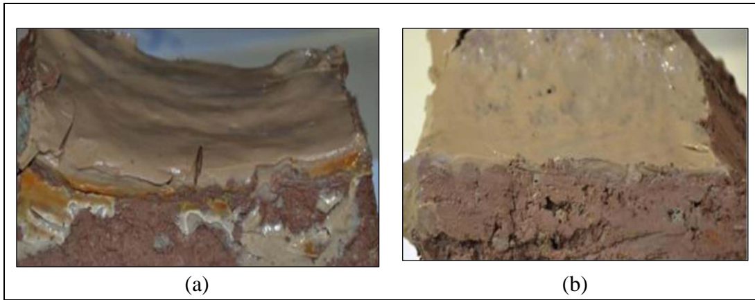
Figure 2. 4: Cross-sectional view of filter cake during a) conventional drilling and b) casing while drilling (Meza et al. 2017).
