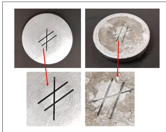
Figure 5. 54: Sealing of a complex fracture with PAM/FNS pill.
