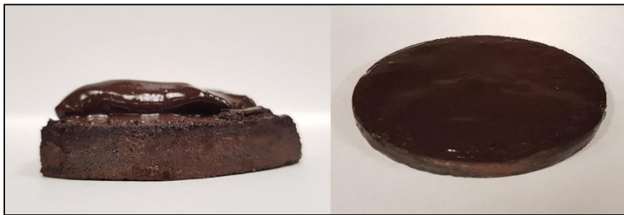
Figure 5. 46: Filter cake on the ceramic disc, calcium carbonate (left), and PBM-25 (right).
