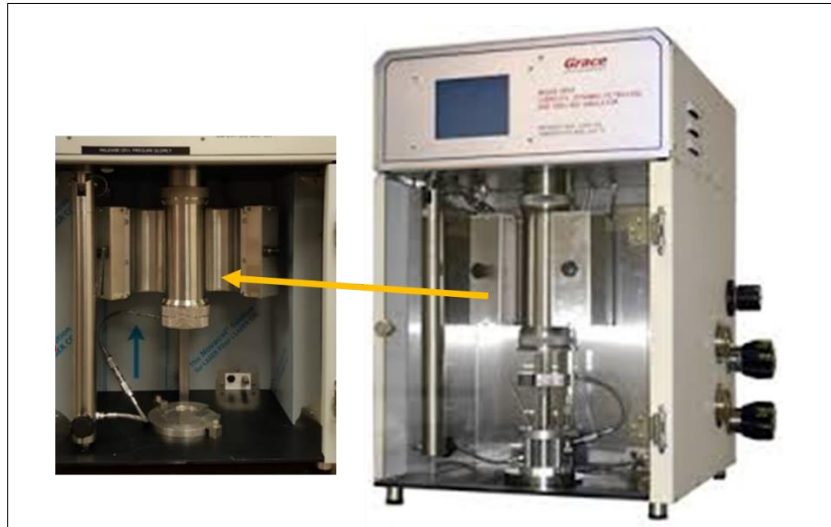
Figure 4. 5: M2200 dynamic drilling simulator, modified after (Ezeakacha and Salehi 2019a).
