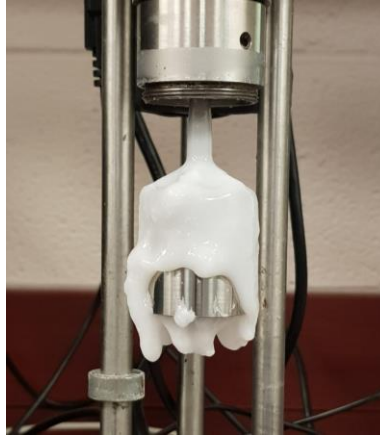
Figure 5. 21: Figure Gel formation on the rotating viscometer pop during the gradual heating.
