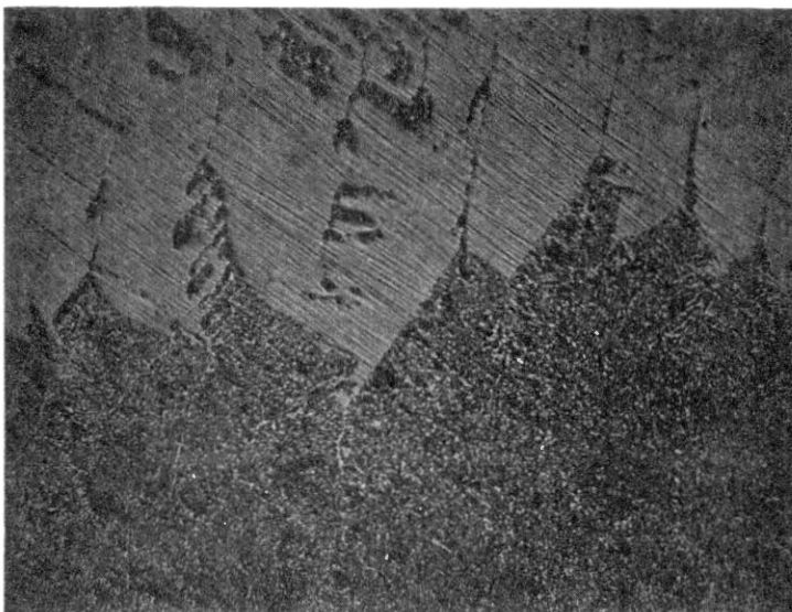
Figure 20. Outward Growing Bismuth Crystals in the Lead-Bismuth Sample. X60
