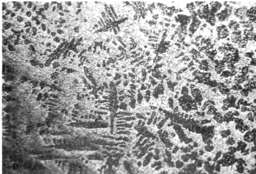
Figure 37. Interface Between the Primary Lead and the Random Lead Dendrites. X60
