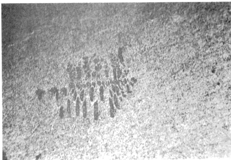
Figure 39. An Independent Lead Dendrite Frozen in the Lead-Tin Eutectic. X60
