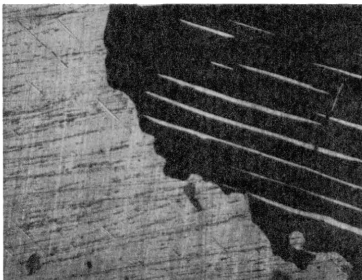
Figure 11. Authentic Tin Structure Obtained by Chemical Removal of the Layers Deformed During Sample Preparation. X50
