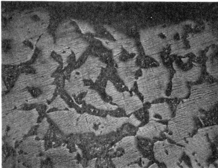
Figure 19. Randomly Packed Bismuth Crystals Found at the Center Surface of the Lead-Bismuth Sample. X60
