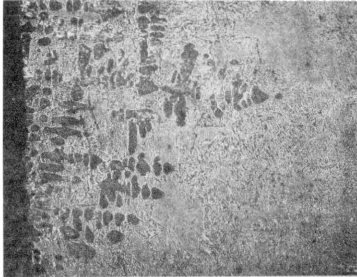
Figure 33. Tin Dendrites at the Inner Surface of the Bismuth-Tin Sample. X100
