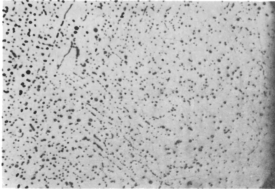
Figure 70. Top Section of a Sample of the Lead-Tin Mixture Showing Reduced Lead Composition There. T_b = 180^\circ\text{C} . X60
