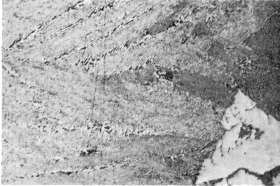
Figure 27. Inward Cellular Growth of the Bismuth-Cadmium Eutectic. X60
