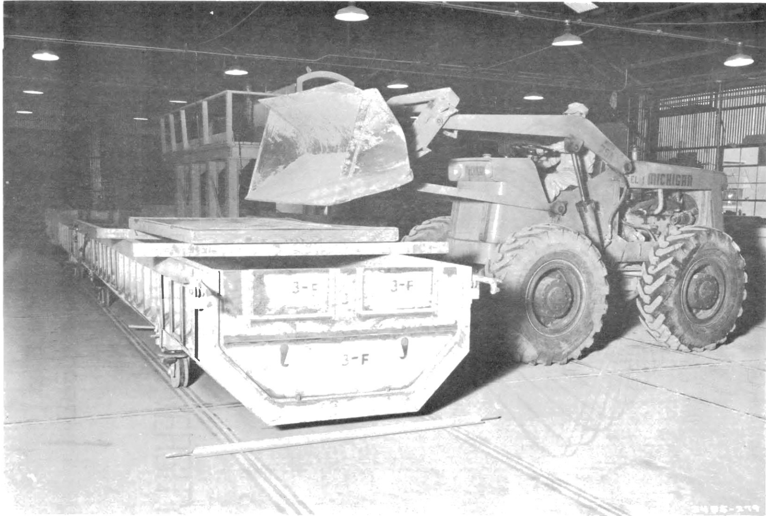
Figure 3.7. Front-end Loader Spreading Sand on Screen During Filling of Soil Bins.
