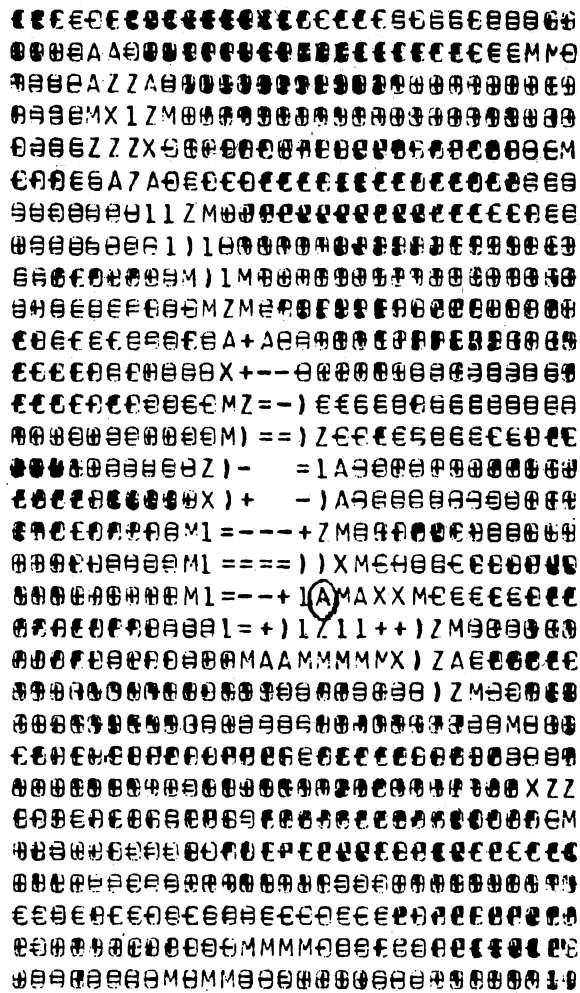
Figure 4. Grey Scale Representation of a Typical Ground Control Point Used in Registration. Plot is From the September Day Scene. A Thermal Contrast of \sim 7^{\circ}\text{C} and \sim 4^{\circ}\text{C} Respectively Exists Between the Point Utilized (Circled A) and the Adjacent Water and Land Mass
