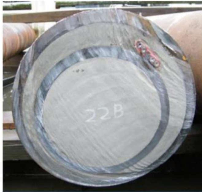
Figure 2.15: Cut test assembly showing complete cement displacement between the casing and tubing. Figure modified from Aas et al. (2016).
