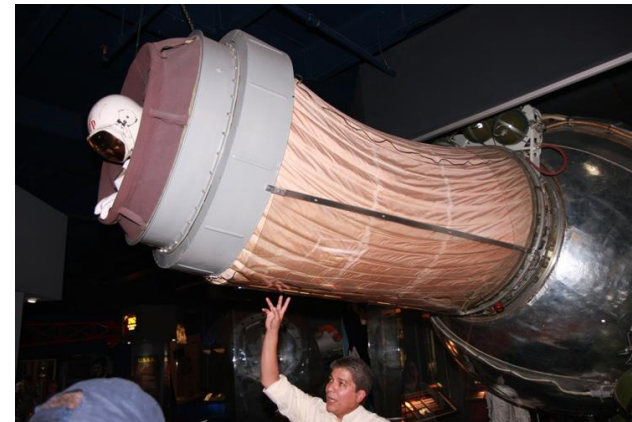
Volga – Soviet Era Crewlock used for first spacewalk
