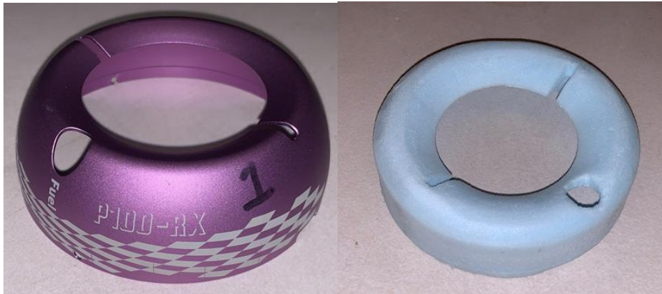
Figure 25. Original Inlet Cowling (Left) and New Inlet Cowling (Right)
