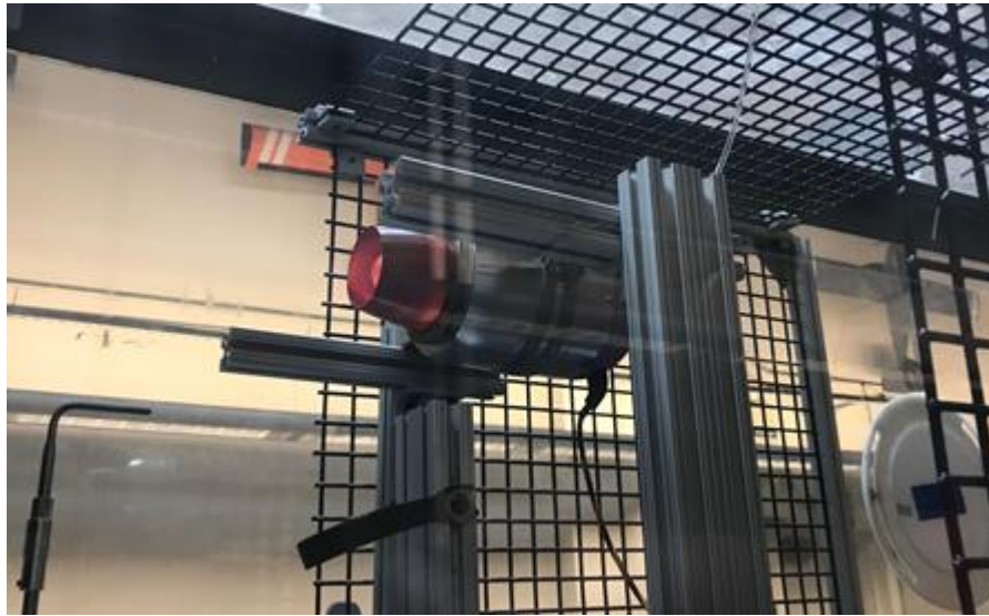
Figure 17. Thrust Stand in Wind Tunnel
