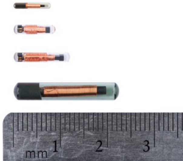
Figure 1.1: Examples of Commercially available RFID PIT Tags that are relatively small [5].
