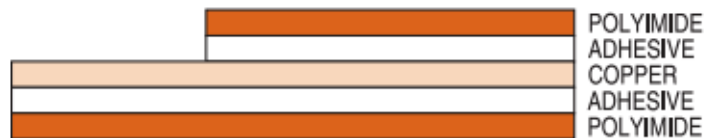
Figure 3.8: Single Layer of Flex Board Material from [24]
