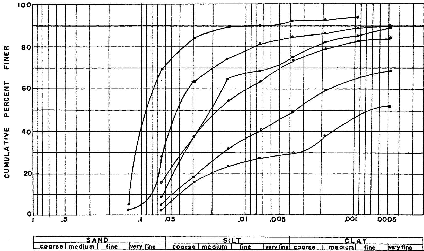
Figure 7. Cumulative Curves of Size Analysis of Sediments
