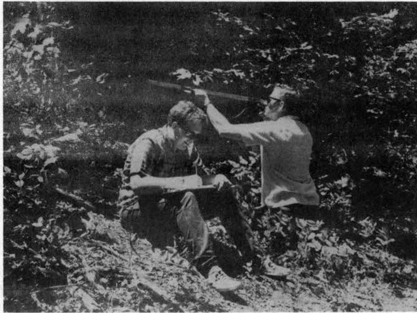
Figure 6. Sampling Overstory Using the Bitterlick-Angle Gauge.
