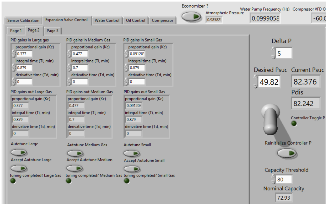
Figure 7.7: Suction pressure control - page two - PID gains
