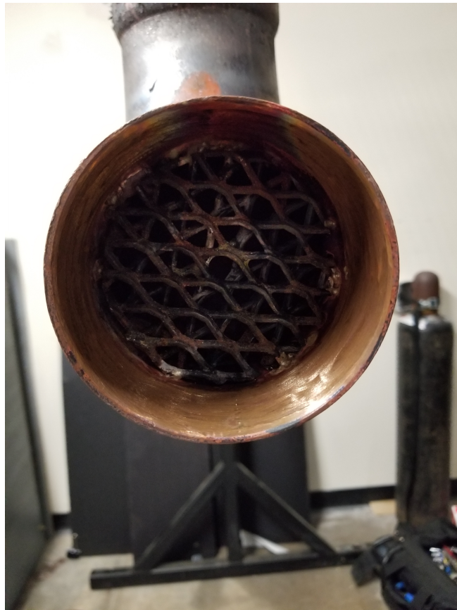
Figure 5.6: Example of expanded metal brazed into a copper elbow
