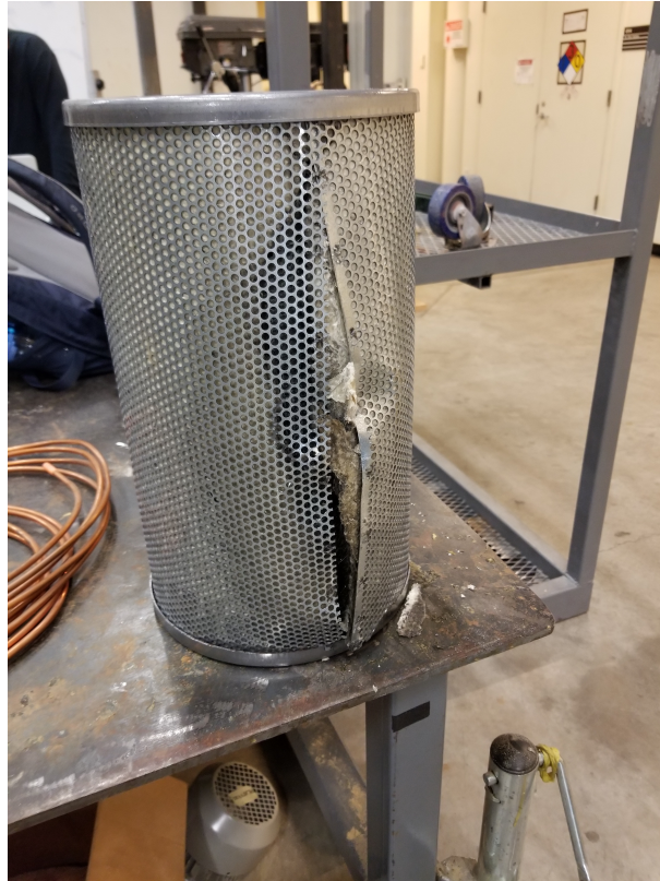
Figure 6.2: Coalescing filter after a blow out caused by too high of an oil carryover rate.
