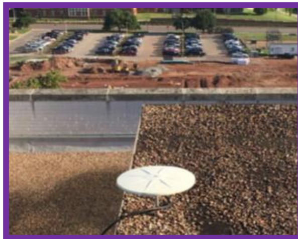
Figure 5. GPS antenna mounted on the building
