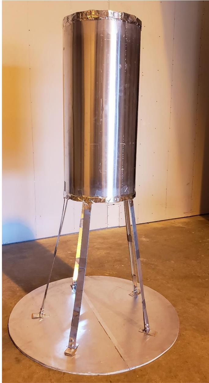
Figure 36: Final Assembly of the Payload and Payload Adapter Models
