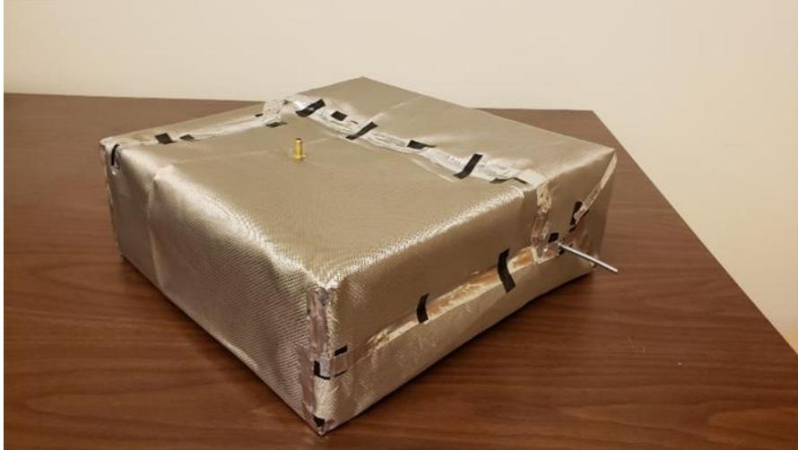
Figure 20: Cu-Ni Fabric Box Modeling the Avionics Box
