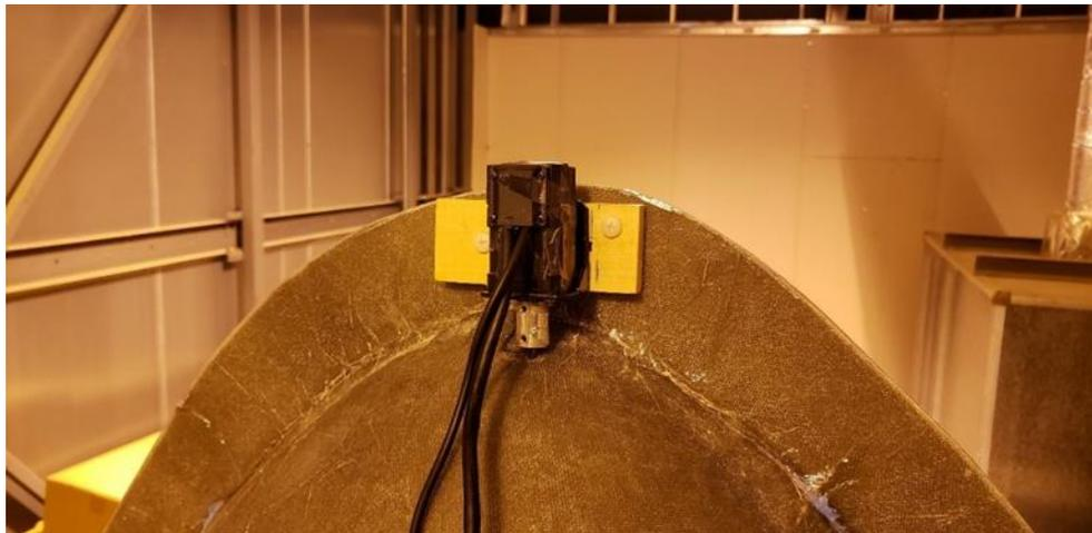
Figure 32: Actual Tuner Assembly Built for the Mechanical Stirrer of the Payload Fairing
