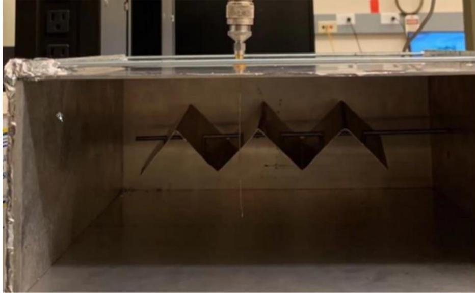
Figure 16: Aluminum Test Box with Front Panel Removed for the Observation of Small Tuner
