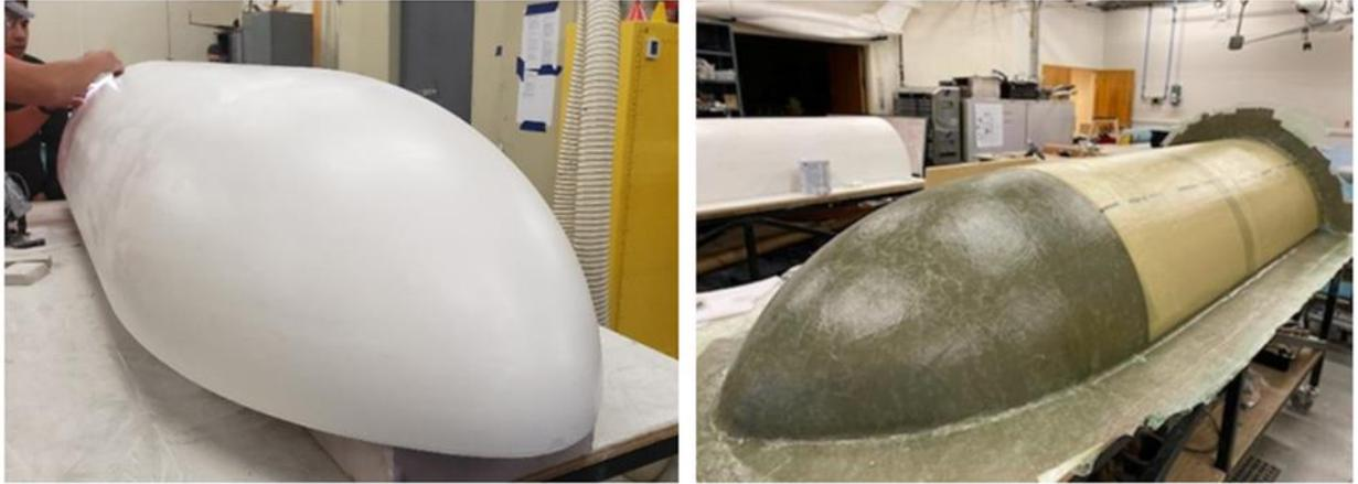
Figure 6: Left figure is the polished mold; right figure is sideview of fabricated fairing half
