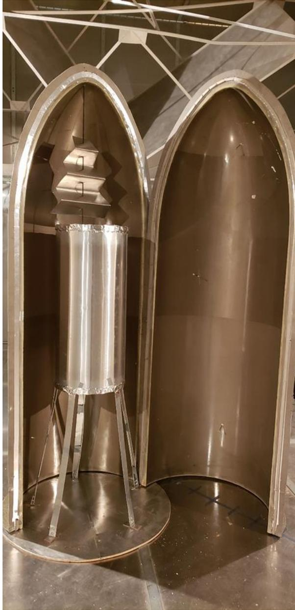
Figure 24: Space Availability within the Payload Fairing Scale Model
