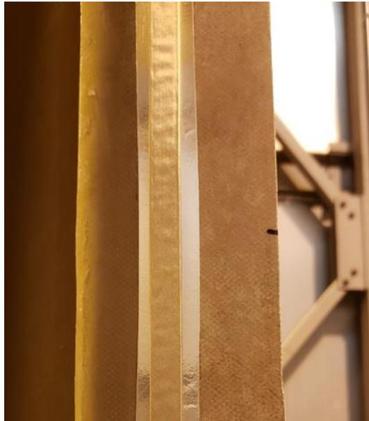
Figure 44: Single Layer of Conductive Adhesive Aluminum Tape for Gasket Conductivity
