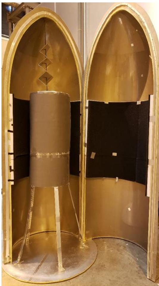
Figure 70: Final Assembly of the Absorbing Foams Installed on the Fairing and Payload
