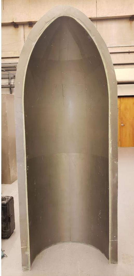
Figure 22: Payload Fairing Half Fabricated by OSU Mechanical & Aerospace Engineering
