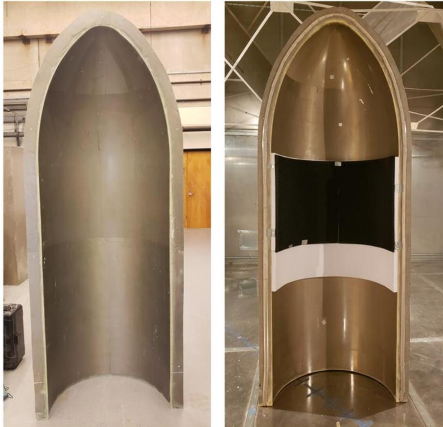
Figure 69: Acoustic Absorbing Foam and RF Absorbing Foam Installed in the Middle Cavity of the Fairing
