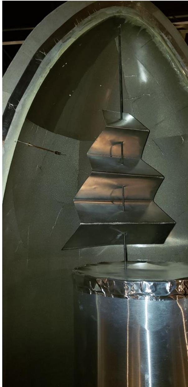
Figure 29: Fairing Tuner Installed in the Top Cavity
