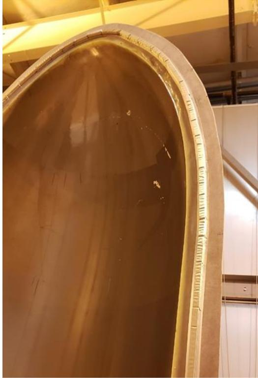
Figure 43: Gaskets Installed on the Fairing Flange
