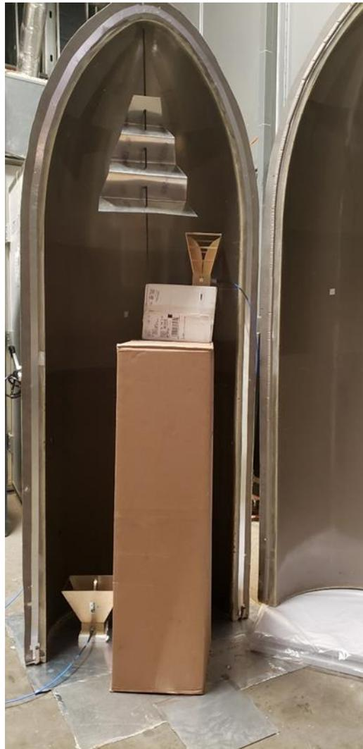
Figure 61: Cardboard Used as Support to Place a Horn Antenna in Top Cavity of the Fairing
