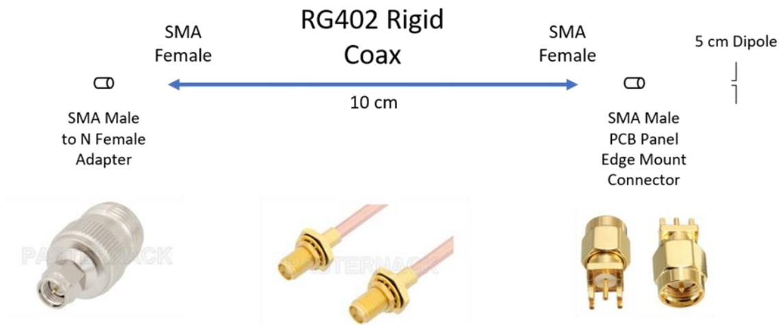
Figure 38: Field Probe Assembly Components
