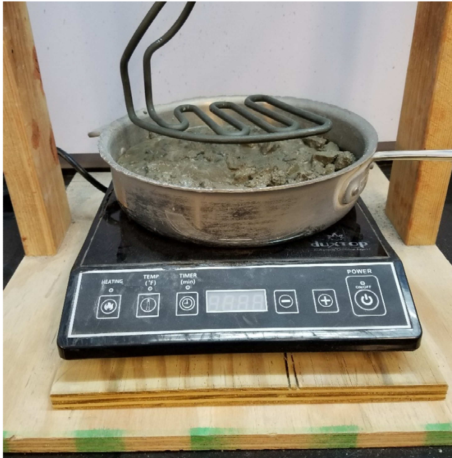
Figure 2-1. Phoenix with dual heating elements for laboratory testing.
