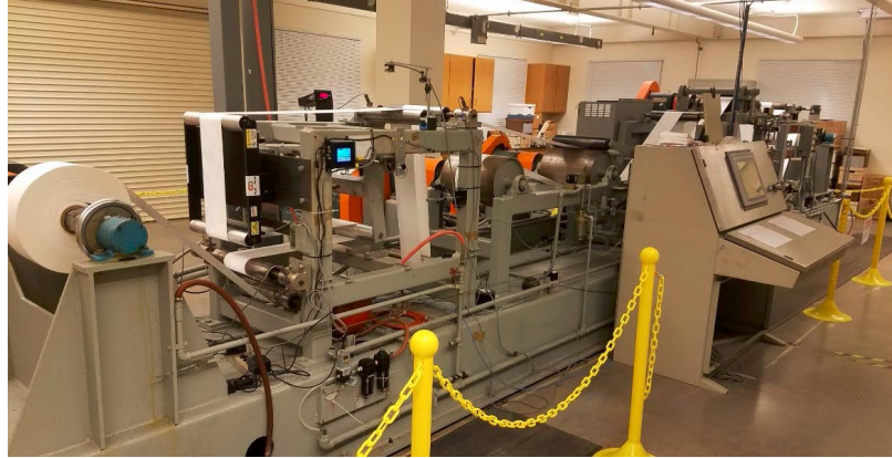
Figure 5.1: Photo of the Euclid Web Line. The unwind section is in the foreground.
