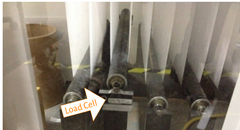
Figure 1.8: Load Cell in Accumulator on HSLT Line
