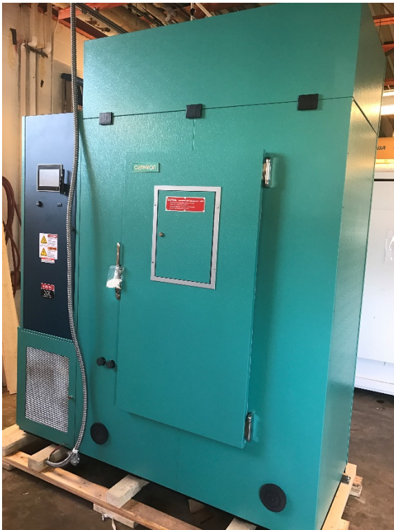
Figure 9. Conviron E8 growth chamber used for the freezing test in Chapter 2 and 3
