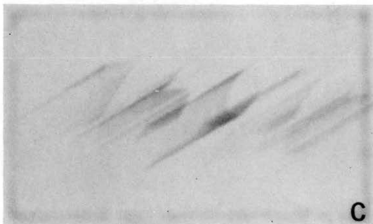
Figure 32. Cross Correlation Between the Hand-Printed Numerals "74074" and a Single Narrow Stripe Inclined at (a) 0, (b) 30, (c) 60 and (d) 90 Degrees
