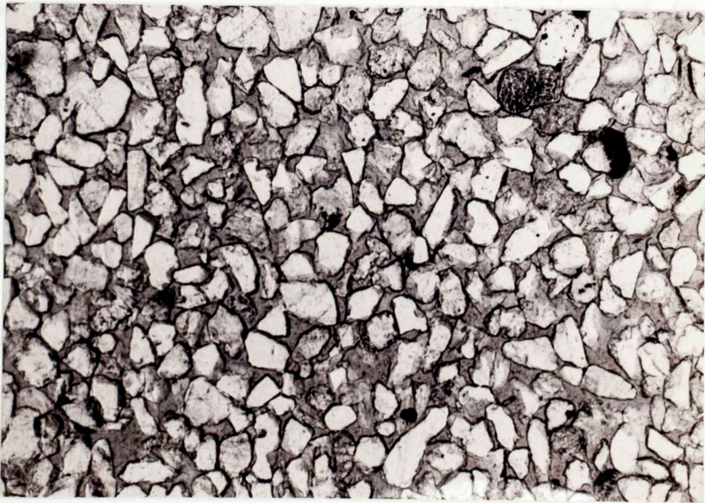
Figure 13. Photomicrographs of undeformed a) Oil Creek Sandstone and b) Antlers Sandstone. The dark colored portions are epoxy filled pore spaces.
