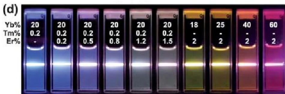
Figure 1.6 NaYF 4 nanoparticles with varied lanthanide ion ratios. Reproduced with permission from reference 59, Copyright Society of Public Analysis. 59
