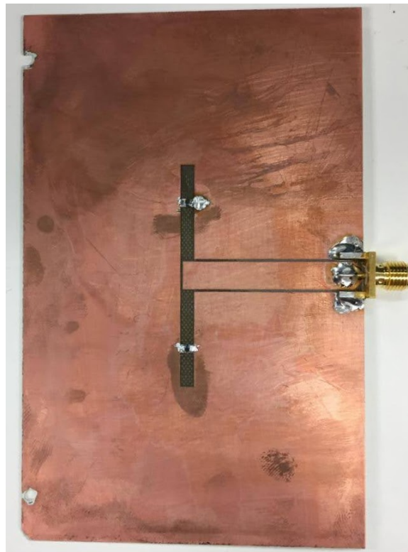
Figure 8.25: Fabricated trap slot antenna with parallel LC loads, 2 nH and 3 pF
