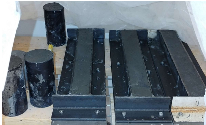
Figure 3.2.3. 3 Cylinder and prismatic molds filled with J3-UHPC
