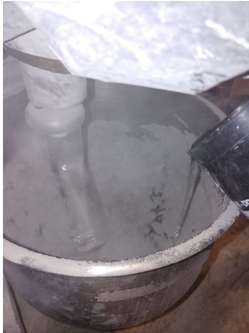
Figure 3.2.2. 3 Adding mixture water to mixing bowl
