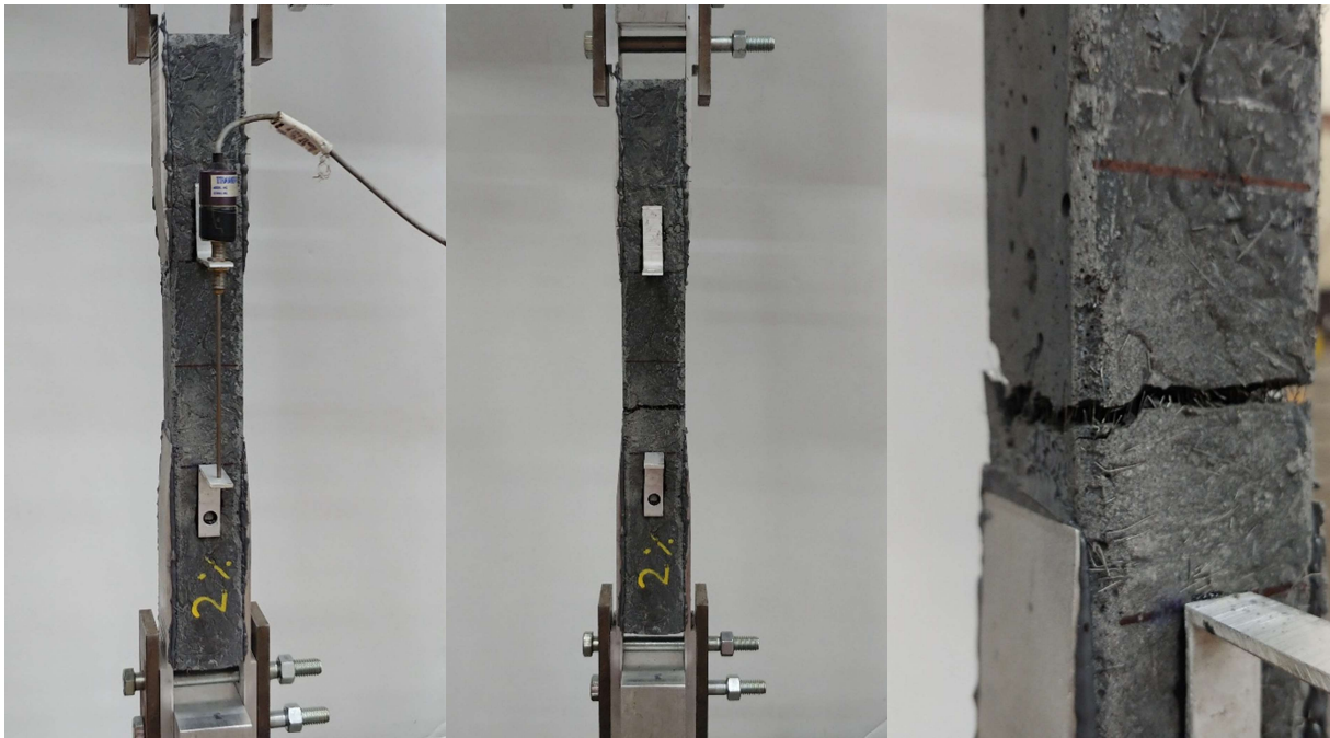
Figure 4.2.2. 9 Crack pattern 2% steel fiber content Specimen 3
