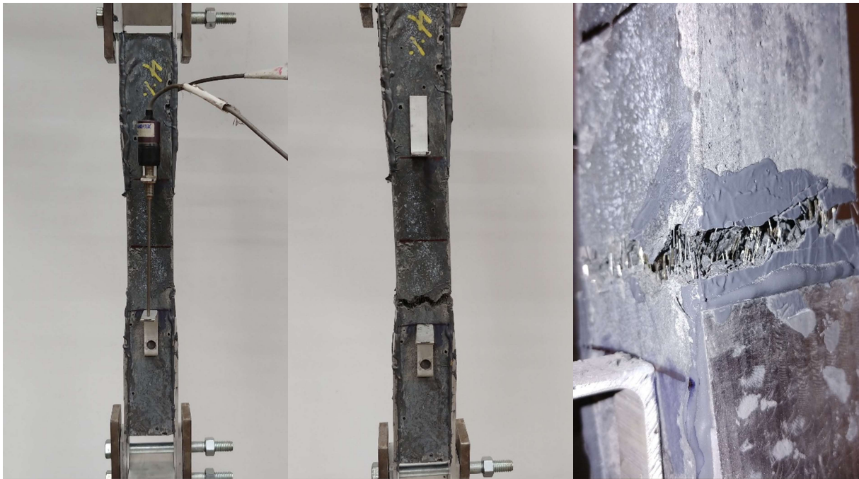
Figure 4.2.2. 12 Crack pattern 4% steel fiber content Specimen 3
