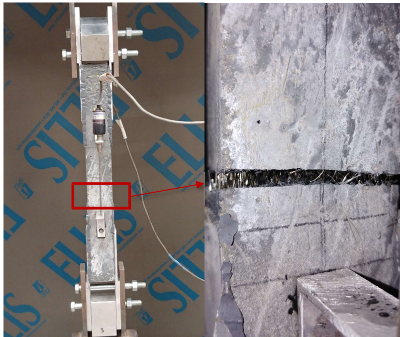
Figure 4.2.2. 4 Crack pattern 1% steel fiber content Specimen 1
