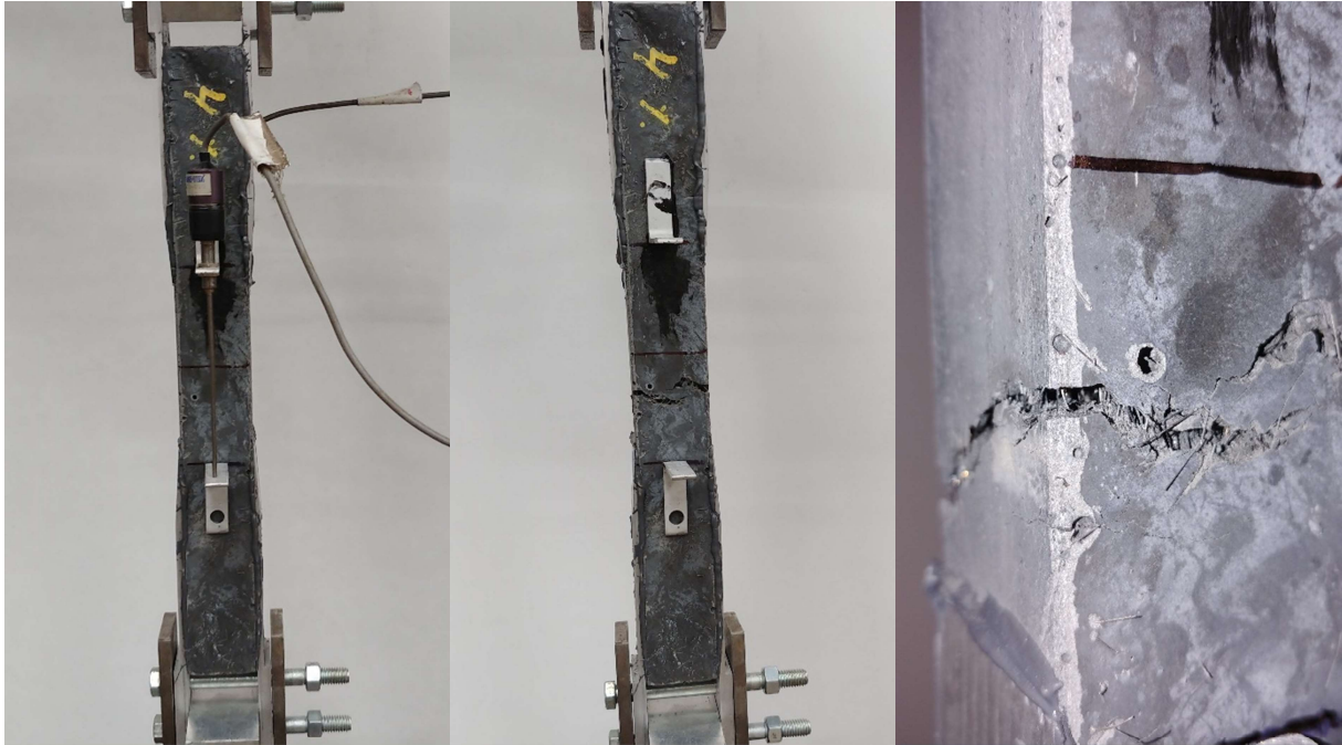
Figure 4.2.2. 11 Crack pattern 4% steel fiber content Specimen 2
