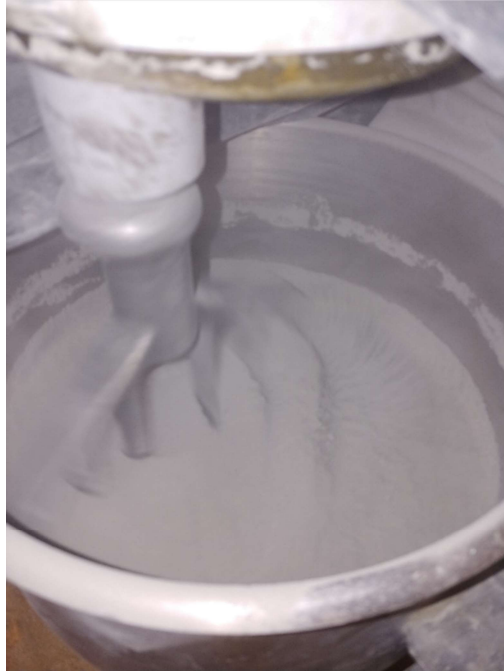
Figure 3.2.2. 1 Mixing of dry J3-UHPC materials
