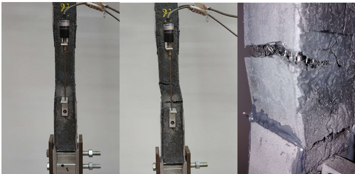
Figure 4.2.2. 7 Crack pattern 2% steel fiber content Specimen 1
