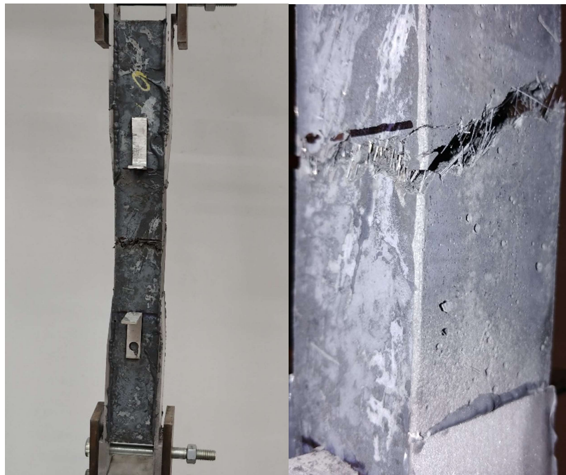
Figure 4.2.2. 13 Crack pattern 6% steel fiber content Specimen 1
