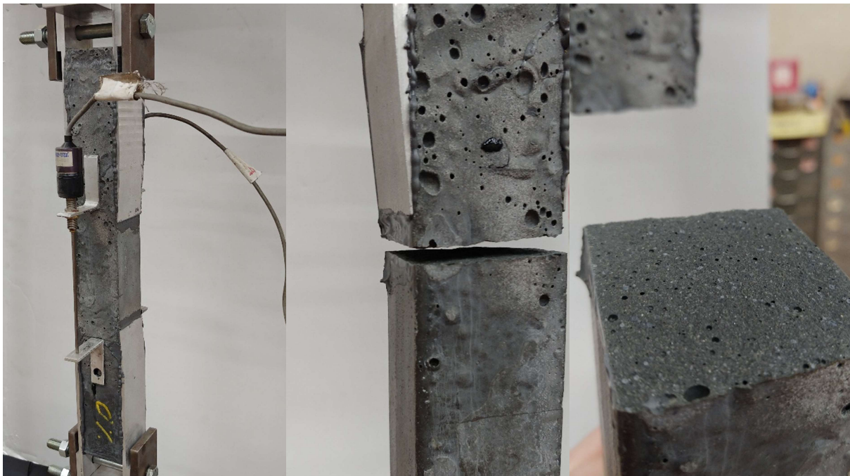
Figure 4.2.2. 1 Crack pattern 0% steel fiber content Specimen 1
