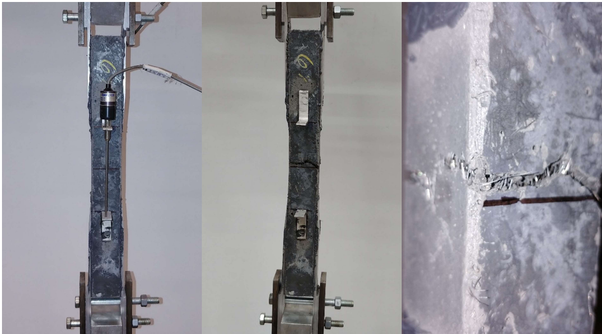
Figure 4.2.2. 15 Crack pattern 6% steel fiber content Specimen 3
