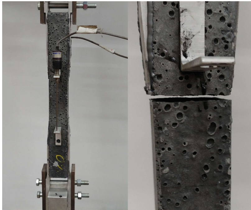
Figure 4.2.2. 3 Crack pattern 0% steel fiber content Specimen 3
