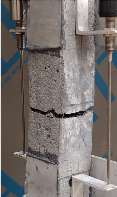
Figure 4.2.2. 5 Crack pattern 1% steel fiber content Specimen 2
