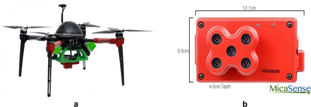
Figure 4.3. Small Unoccupied Aerial System (a) and MicaSense RedEdge multispectral sensor (b)
