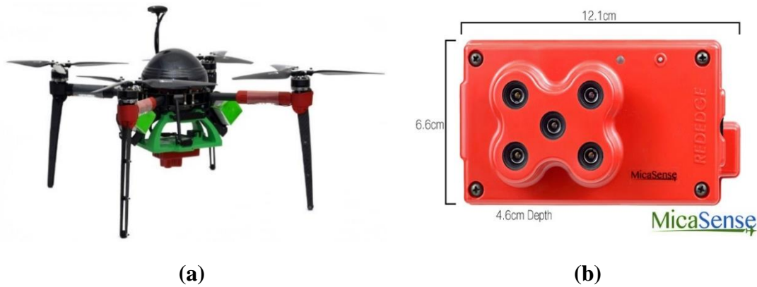
Figure 2.2. Small unnamed aerial system used to collect multispectral data (a) and MicaSense RedEdge multispectral sensor (b).
