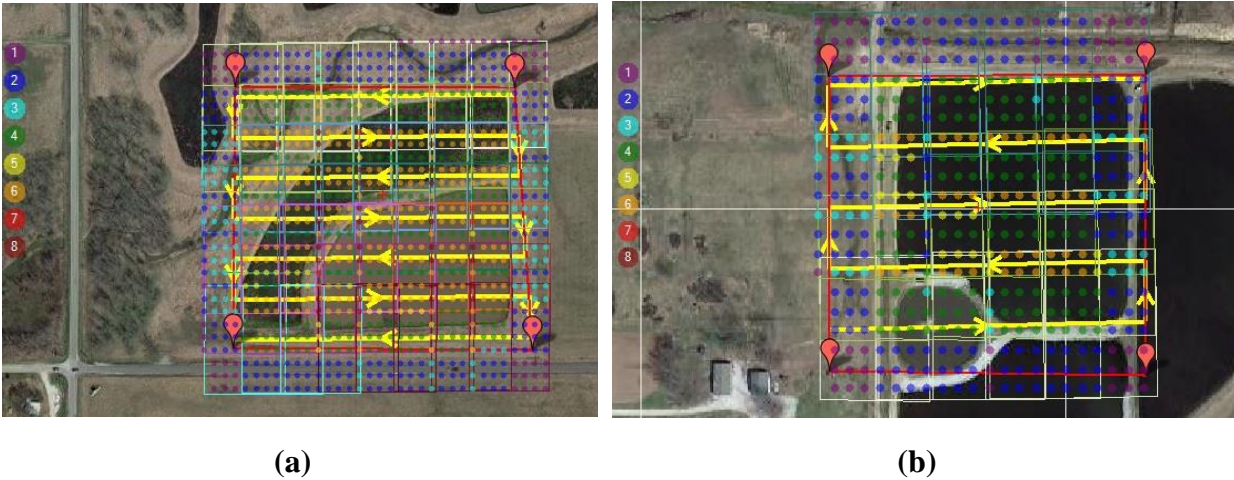
Figure 2.3. Small Unoccupied aerial system (sUAS) flight path (yellow arrow) and imagery footprint (with number of overlapping pictures) at the Nursery Ponds (a) and Wastewater Lagoon (b).
