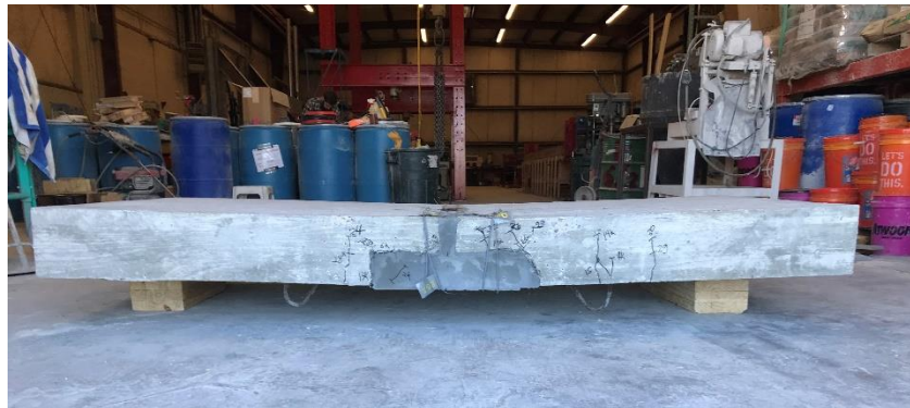
Figure 33: Slab curvature after failure
