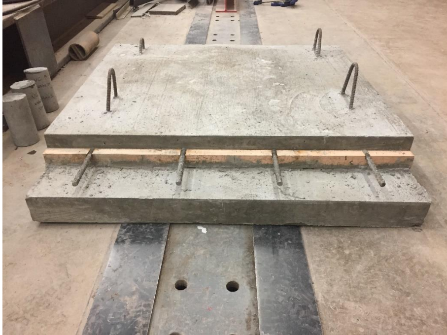
Figure 128: Conventional concrete panel after removing wooden form
