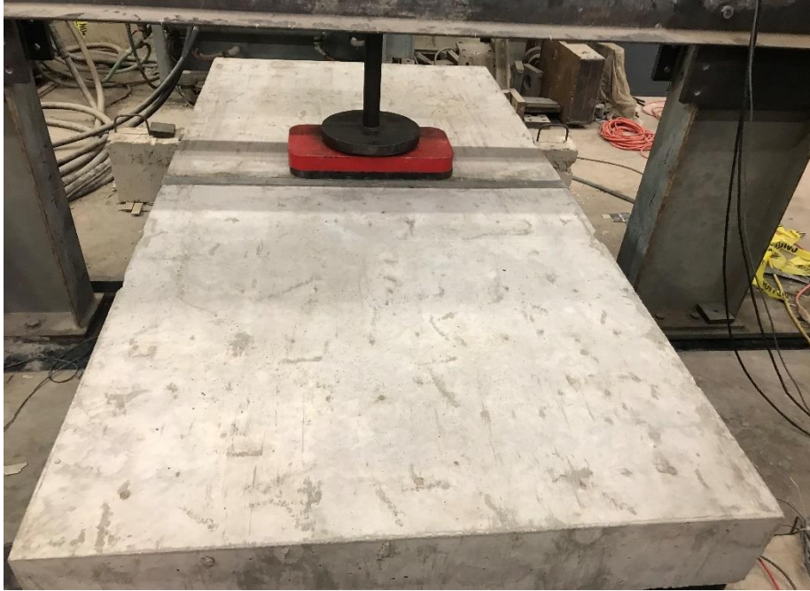
Figure 25: Test setup for slabs using the MTS hydraulic ram
