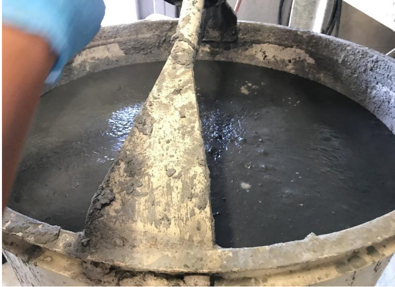
Figure 124: UHPC inside concrete transfer bucket
