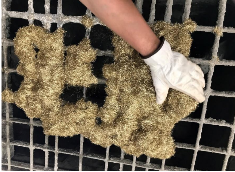
Figure 122: Steel fibers added to UHPC mixture
