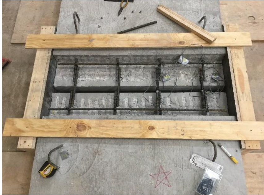
Figure 19: Two slab panels with formwork in place and strain gauges installed
