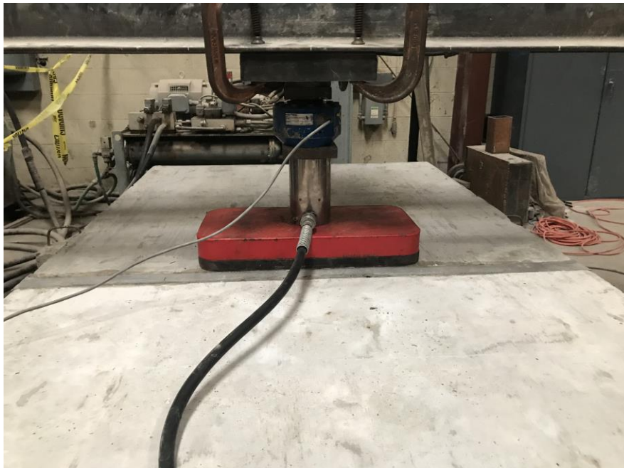
Figure 26: Test setup for slabs using the manually controlled hydraulic cylinder and pump
