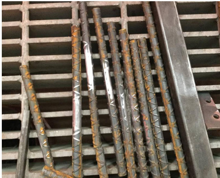
Figure 18: Splice bars ready for strain gauge installation
