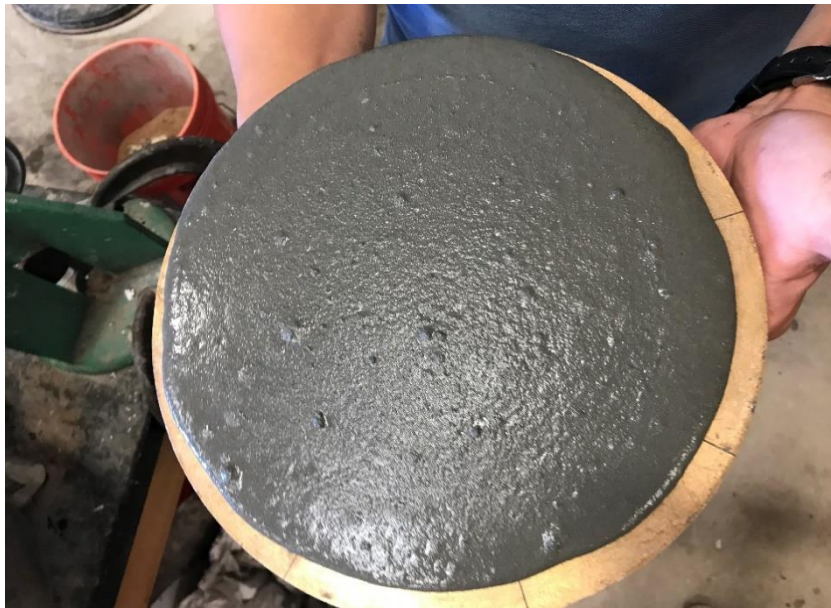
Figure 125: UHPC flow test using mortar flow table
