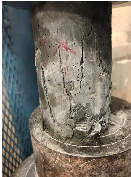
Figure 127: UHPC cylinders after compressive strength test
