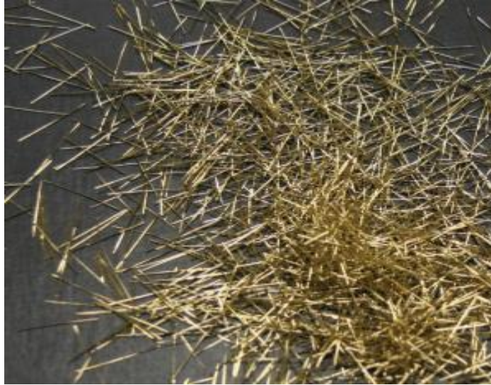
Figure 3: Typical steel fiber reinforcement (Graybeal 2014)
