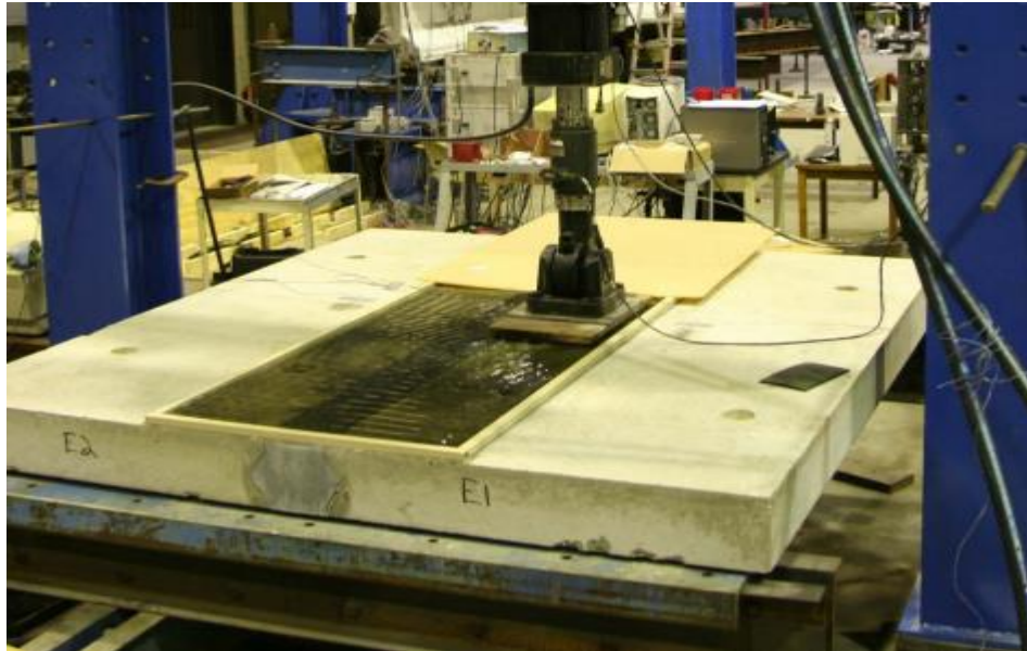
Figure 5: Cyclic test setup for longitudinal UHPC connection (Graybeal 2010)
